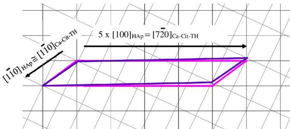
**Figure SI3:** A new 2D-coincidence cell obtained by rotating the  $[100]_{\text{Ca-Cit-TH}}$  vector clockwise by  $25^\circ$  with respect to the  $[100]_{\text{HAp}}$  vector, while the common origin is maintained.
