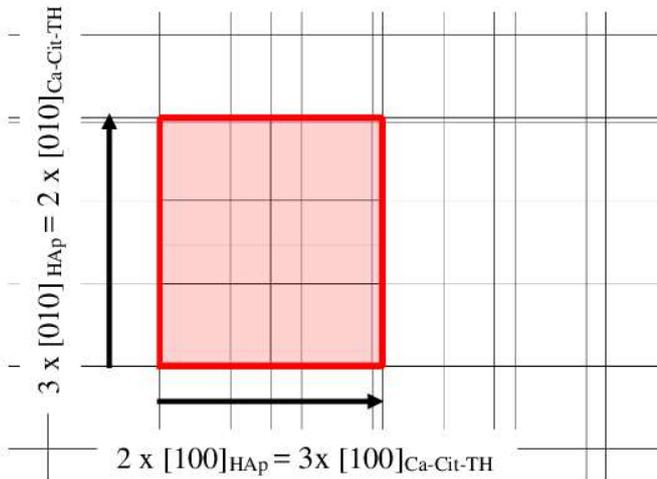
**Figure SI2:** 2D coincidence cell between the (001) cell of HAp and the (001) cell of Ca-Cit-TH as reported in Figure SI1.
