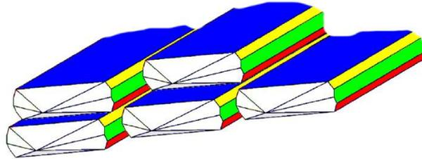
**Figure SI4:** Double fence-like aggregate of Hap crystals welded on both the  $\{10\bar{1}\}$  (better visible on the left) and the  $\{001\}$  faces (better visible on the right) and their reciprocal arrangement sketched in the scheme below.
