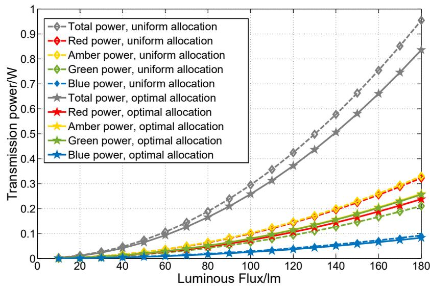
**Figure 5.** Transmission power comparison between the proposed optimal power allocation strategy and the uniform power allocation method with interference coefficient  $\tau = 0.05$  under CCT = 5700 K.
