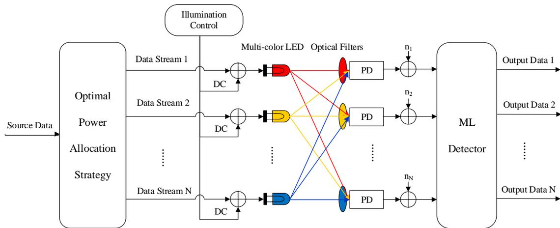
**Figure 1.** CMIMO model for the multi-color light-emitting diodes (LED) based visible light communication (VLC) system.
