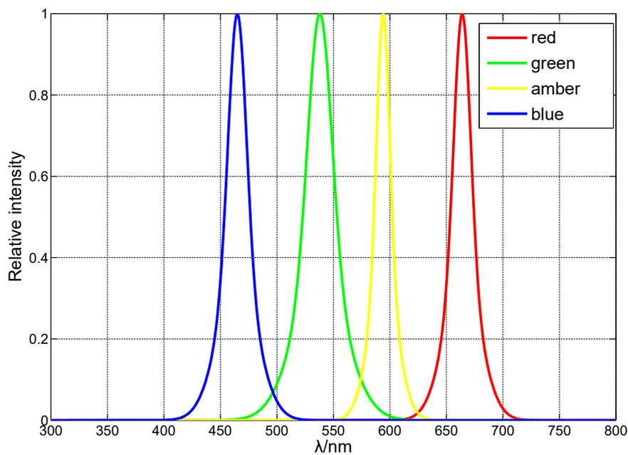
Figure 2. Spectral model for the quadrichromatic LED (QLED) with red/amber/green/blue (RAGB) colors.
