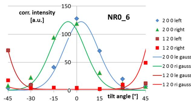
**Figure 7.** Intensities of the crystalline peaks of the sample NR0 with a stretch ratio of 6:1 in dependence of sample rotation, measured values (symbols) and values of the model (continuous lines) in analogy to Figure 5.
