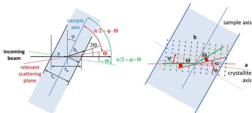
**Figure 4.** Detailed scattering geometry (here for the reflection (1 2 0): The sample is rotated by an angle  $\psi$  to the beam, the *a*-axis of an individual crystallite has an angle of  $\varphi$  within the sample, the scattering crystalline plane has an angle of  $\alpha$  to the *a*-axis. The scattering angle  $\Theta$  is between the incoming beam and the scattering plane as well as between this and the scattered beam.
