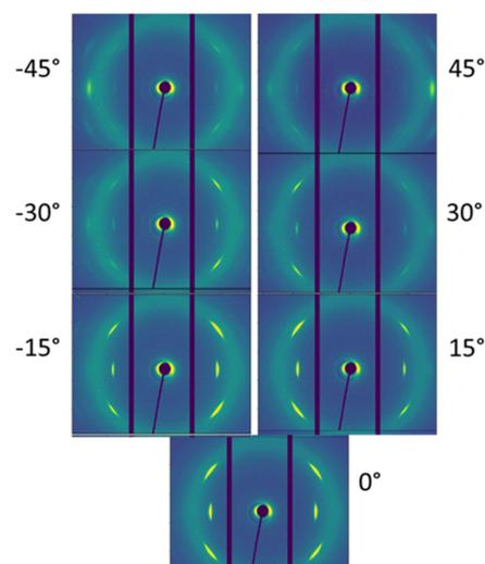
**Figure 3.** Patterns of the sample NR0\_5 after intensity-, thickness- and tilt-correction in dependence of the angle of rotation of the sample around the tensile axis, which is vertical. Rotation angle  $\pm 45^\circ$ ,  $\pm 30^\circ$ ,  $\pm 15^\circ$ ,  $0^\circ$  (from top to bottom, in a.u.).
