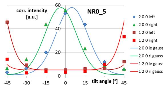
**Figure 6.** Measured intensities of the crystallite peaks (symbols) and model of the intensities using a Gaussian distribution superimposed to certain randomly distributed crystallites for the orientation distribution of crystallites in the unfilled stretched natural rubber with a stretch ratio 5:1, NR0\_5, parameters in Table 1 (continuous lines).
