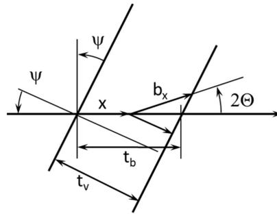
**Figure 2.** Sketch for the correction of different beam paths within the sample due to the tilted sample orientation with a tilting angle  $\psi$  between incoming beam and sample. Instead of the initial thickness  $t_v$  of the sample the beam passes the thickness  $t_b$ , while the path of the scattered beam is  $x + b_x$ .
