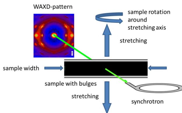
**Figure 1.** Arrangement of the stretched sample in the beam of the synchrotron source. The equatorial reflections have the indices (2 0 0) and (1 2 0), here a pattern of a fiber symmetrical sample is shown.
