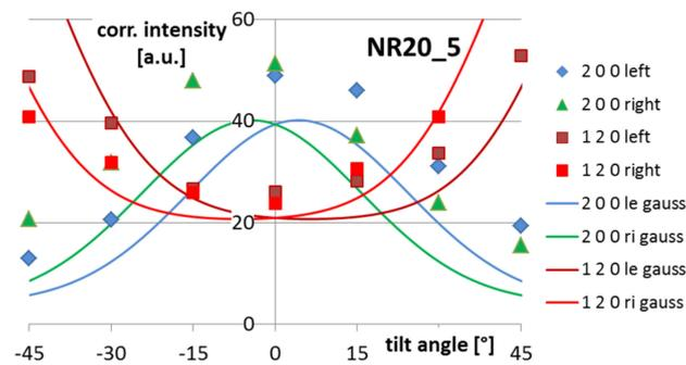
**Figure 8.** Intensities of the crystalline peaks of the sample NR20 with a stretch ratio of 5:1 in dependence of sample rotation, measured values (symbols) and values of the model (continuous lines) in analogy to Figure 5.
