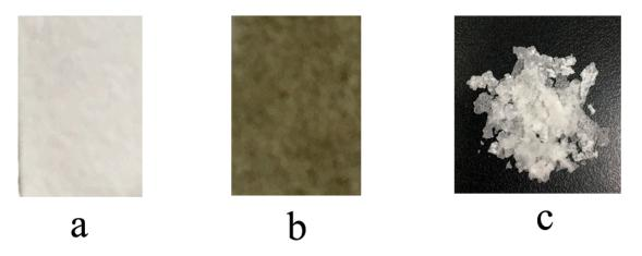
**Figure 5.** Photographs of (a) Cell-SH paper before used as reducing agent; (b) Cell-SH paper after used as reducing agent; and (c) final PMMA obtained from hetrogeneous AGET ATRP with Cell-SH as reducing agent in the present of a limited of air. Polymerization conditions:  $[MMA]_0/[EBPA]_0/[CuBr_2]_0/[PMDETA]_0 = 400/1/0.25/0.5, m_{[Cell-SH]} = 50 mg.$
