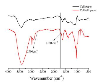
Figure 1. FT-IR spectra of (a) pristine cellulose paper; and (b) cellulose paper grafted with thioglycolic acid.
