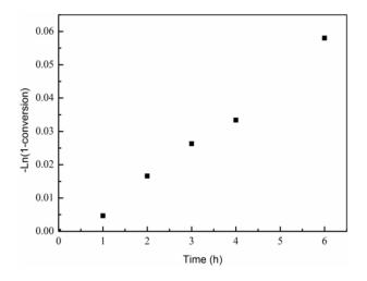
**Figure 2.** Semilogarithmic kinetic plots for photoinduced Cu(II)-mediated RDRP of AN in DMSO with P(VDF-*co*-CTFE) as macroinitiator ([Cl]:[Cu]:[L]:[AN] = 1:(1/32):(6/32):30, UV ( $\lambda_{max}$  = 365 nm).
