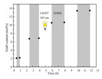
**Figure 1.** Graft contents vs. reaction time dependence for photoinduced Cu(II)-mediated RDRP of AN in DMSO with P(VDF-*co*-CTFE) as macroinitiator under "on-off" light sequence ([Cl]:[Cu]:[L]:[AN] = 1:(1/32):(6/32):30, UV ( $\lambda_{max} = 365$  nm)).
