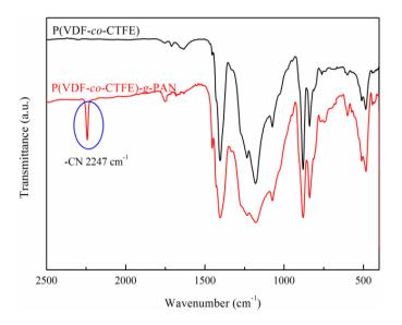
**Figure 3.** Fourier transform infrared (FTIR) spectrum of pristine P(VDF-*co*-CTFE) and P(VDF-*co*-CTFE)*g*-PAN (Table 1, run 5).
