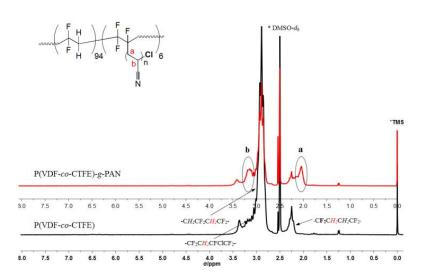
Figure 4. <sup>1</sup>H NMR of pristine P(VDF-co-CTFE) and P(VDF-co-CTFE)-g-PAN (Table 1, run 5).
