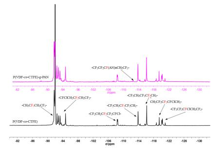
Figure 5. <sup>19</sup>F NMR of pristine P(VDF-co-CTFE) and P(VDF-co-CTFE)-g-PAN (Table 1, run 5).
