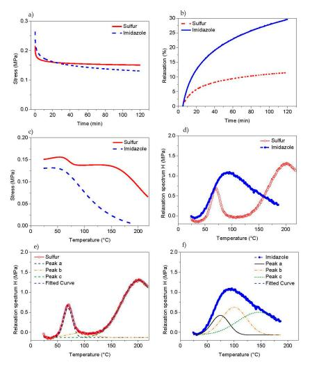
**Figure 4.** Isothermal relaxation test at 23 °C; (**a**) stress at constant strain (stretching ratio  $\lambda$  = 1.5); (**b**) stress relaxation as a function of time. Non-isothermal relaxation test; (**c**) stress vs. temperature curves and (**d**) relaxation spectra. De-convoluted relaxation spectra of (**e**) sulphur cured BIIR and (**f**) imidazole modified BIIR.
