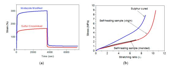
**Figure 3.** (**a**) Stretching experiment of the modified BIIR and the mended sample. The mended sample was previously cut half of the width and allowed to heal for 1 h; (**b**) Creeping experiment of the sulphur vulcanized and modified BIIR rubbers.
