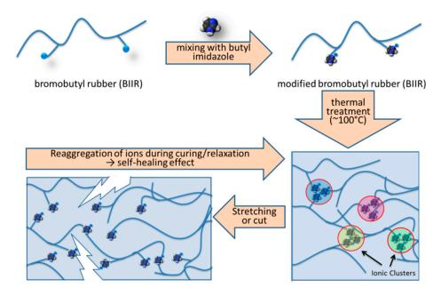
**Figure 1.** Schematic presentation of modification of bromo-butyl rubber (BIIR) by butyl imidazole. The ionic imidazolium bromide group can be associated together to form a crosslinked-type network structure. This network is broken during damage and rebuild during healing.
