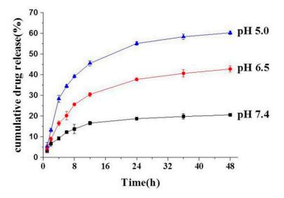
**Figure 6.** DOX release profiles of mPEG-PCL-Imi-DOX micelles under different pH levels. Data were presented as mean  $\pm$  standard deviation (SD) (*n* = 3).
