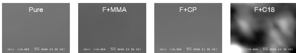
Figure S2 SEM images of PMMA hybrids containing POSS fillers (2 mol%). Scale bars represent 1 \mu\text{m} .
