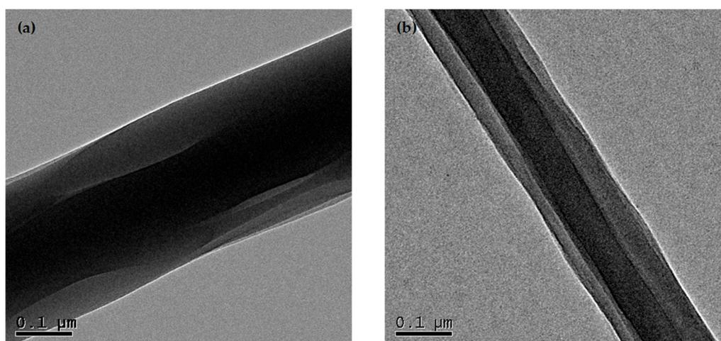
**Figure 4.** TEM photographs of the TPP loaded core-shell fibers with the different weight ratios (DCM/DMF) ((a) 9:1; (b) 5:5) at core solution flow rate of 0.2 mL/h.
