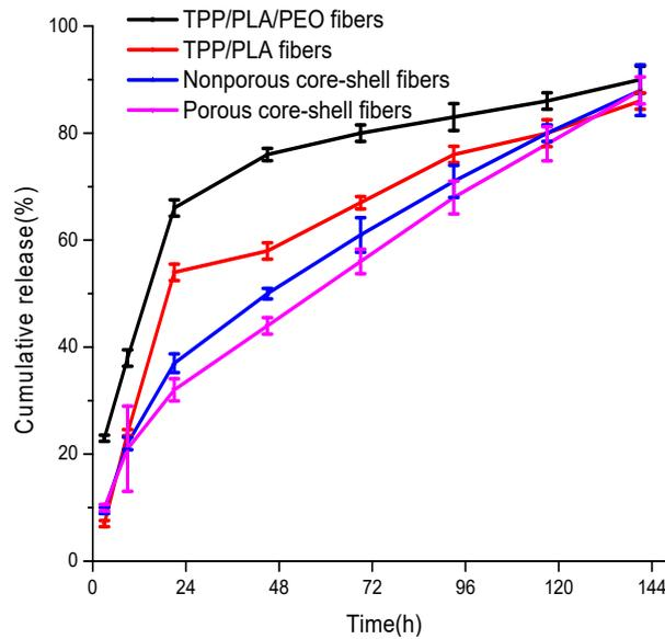
**Figure 7.** TPP release profiles from porous core-shell, nonporous core-shell, PLA, and PLA/PEO fiber membranes loaded with TPP.
