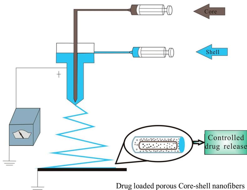
**Figure 1.** Schematic diagram of the coaxial electrospinning setup.
