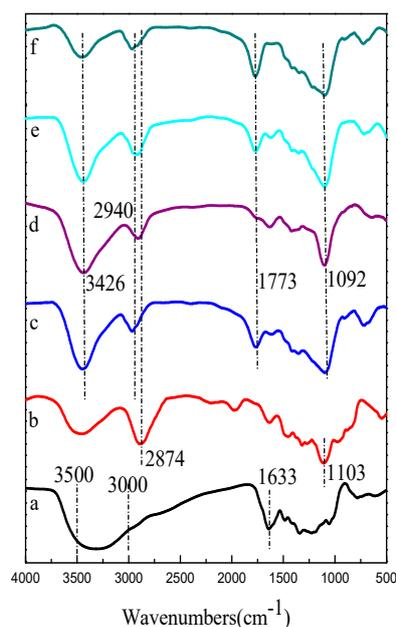
**Figure 5.** FTIR spectra of TPP (a); PEO (b); PLA (c); and core-shell fibers with the different weight ratios (DCM/DMF) ((d) 9:1; (e) 7:3; (f) 5:5) at core solution flow rate of 0.2 mL/h.
