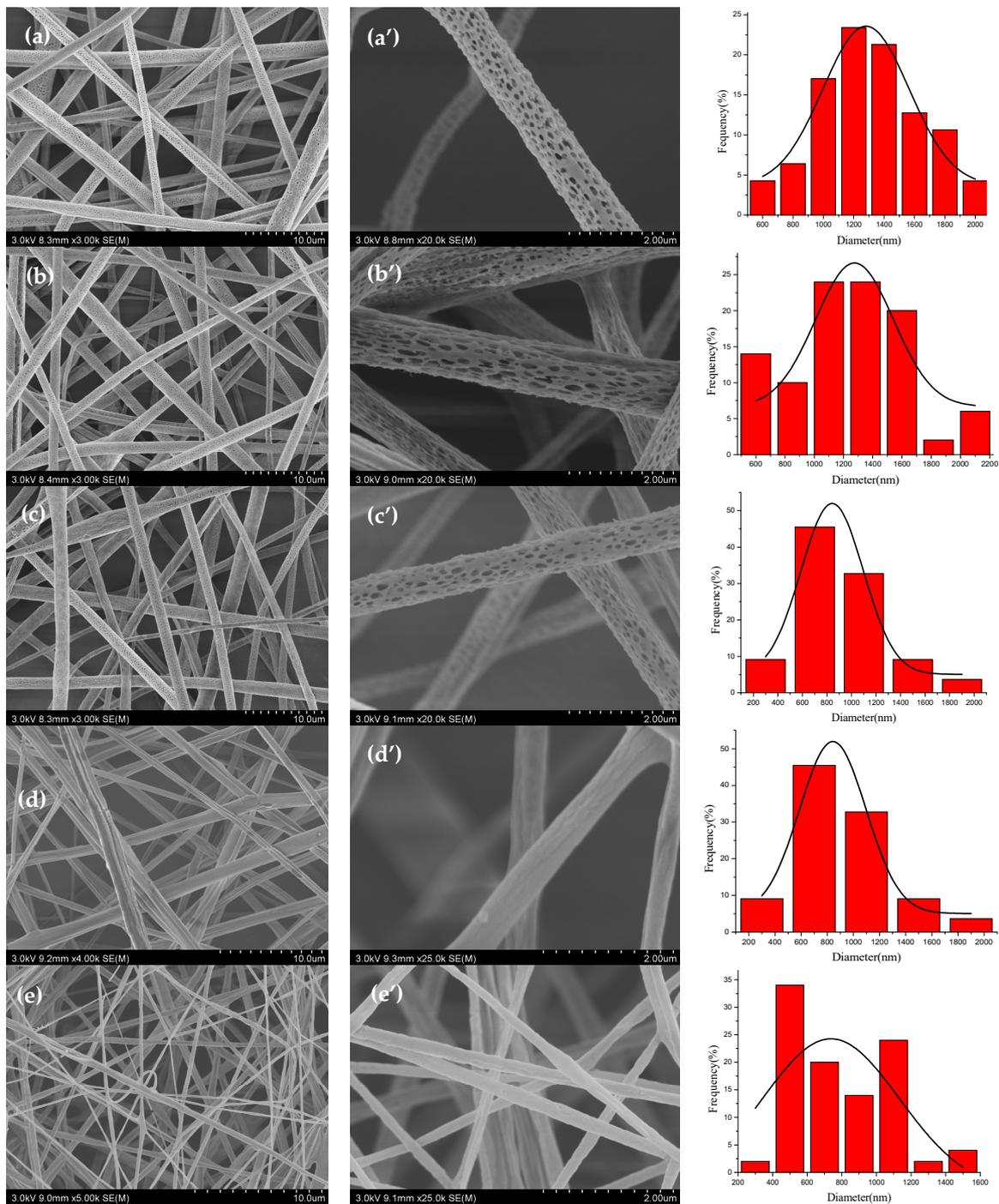
**Figure 2.** SEM pictures of tea polyphenol (TPP) loaded porous core-shell fibers with the weight ratio 9:1 at core solution flow rates of (a,a') 0.05 mL/h; (b,b') 0.1 mL/h; and (c,c') 0.2 mL/h, respectively, and nonporous core-shell fibers at core solution flow rates of 0.2 mL/h with the weight ratio (DCM/DMF) (d,d') 7:3 and (e,e') 5:5. The rightmost figures were the according diameter distribution.
