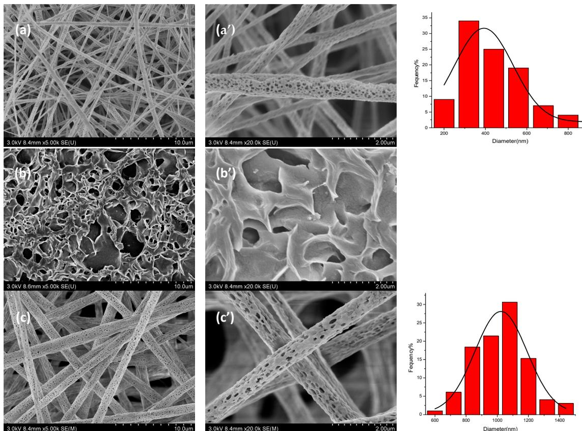
Figure 3. SEM pictures of electrospun porous TPP/ poly(lactic acid) (PLA) (a,a’), TPP/ polyethylene oxide (PEO) (b,b’) and TPP/PLA/PEO (c,c’) fibers. The rightmost figures were the according diameter distribution.
