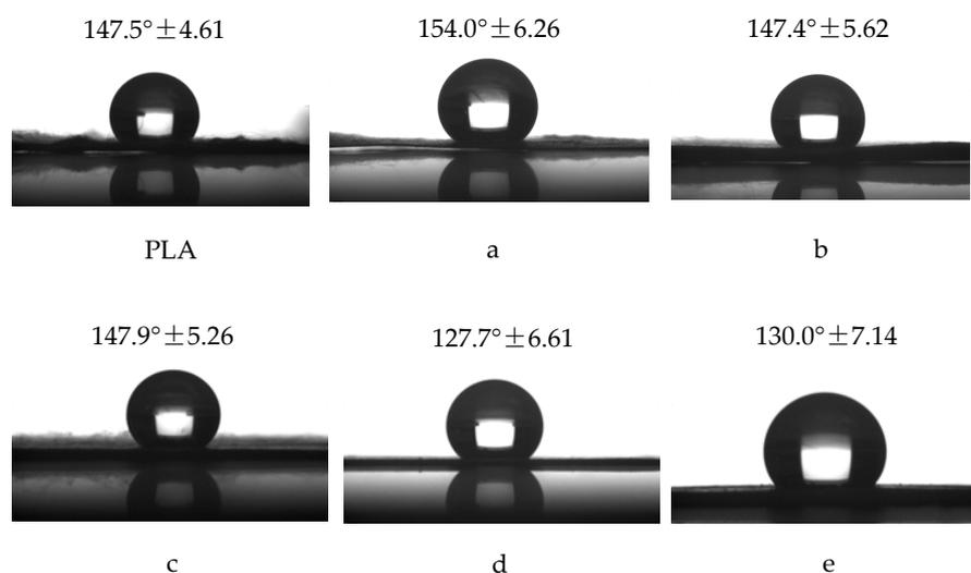
**Figure 6.** Static contact angle of PLA fibers, porous core-shell fibers with the weight ratio 9:1 at core solution flow rates of (a) 0.05 mL/h; (b) 0.1 mL/h; and (c) 0.2 mL/h, respectively, and nonporous core-shell fibers at core solution flow rates of 0.2 mL/h with the weight ratio (DCM/DMF) (d) 7:3 and (e) 5:5.
