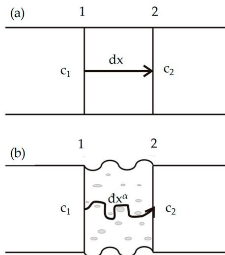
**Figure 8.** Schematic diagrams of Fickian diffusion of drug from (a) nonporous fibers and (b) porous fibers.
