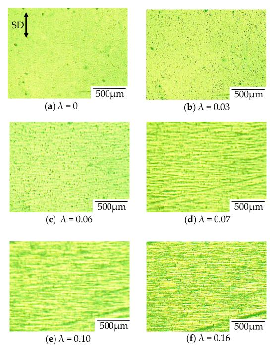
Figure 8. In situ observation for void formation of OD-PC during stretching under  $CO_2$  at 5 MPa.
