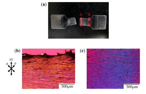
**Figure 6.** Photograph and polarized optical micrographs of OD-PC obtained by stretching under CO<sub>2</sub> at 5 MPa. (**a**) Photograph of the fractured specimen; (**b**) Polarized optical micrograph for region A; and (**c**) Polarized optical micrograph for region B.
