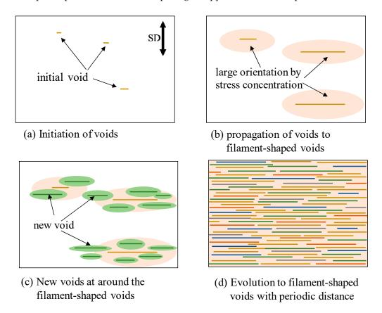
**Figure 11.** Schematic illustration for the evolution of a filament-shaped porous structure of OD-PC by stretching under CO<sub>2</sub>.
