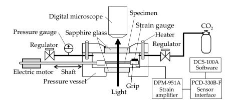
**Figure 1.** Schematic illustration of a stretching instrument for tensile-deformation measurements and in situ observation under high-pressure CO<sub>2</sub>.
