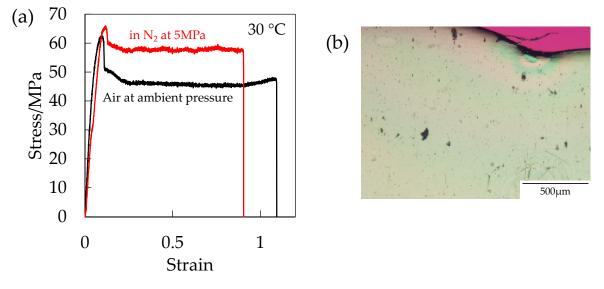
**Figure 14.** (a) Stress–strain curve of OD-PC under N<sub>2</sub> at 5 MPa and under air at atmospheric pressure; (b) polarized optical micrographs of OD-PC obtained by stretching under N<sub>2</sub> at 30 °C.
