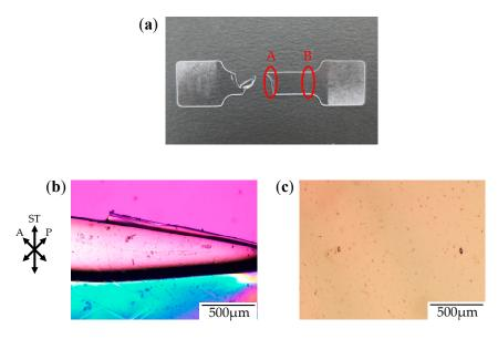
**Figure 13.** Photograph and polarized optical micrographs of OD-PC obtained by stretching  $CO_2$ -absorbed PC under air at atmospheric pressure at 30 °C after absorbing and releasing  $CO_2$  at 5 MPa: (a) Photograph of fractured specimen; (b) Polarized optical micrograph for region A; and (c) Polarized optical micrograph for region B.
