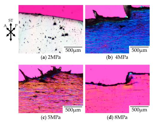
**Figure 5.** Polarized optical micrographs of stretched-and-fractured OD-PC obtained by stretching at  $30 \degree C$  under CO<sub>2</sub> of various pressures.
