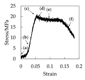
Figure 7. Stress-strain curve of OD-PC during stretching under CO<sub>2</sub> at 5 MPa.
