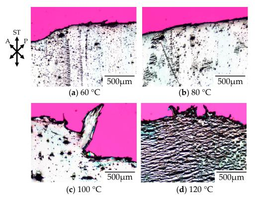
**Figure 2.** Polarized optical micrographs of stretched-and-fractured low molecular weight polycarbonate for optical disc grade (OD-PC) obtained by stretching under atmospheric pressure at various temperatures.
