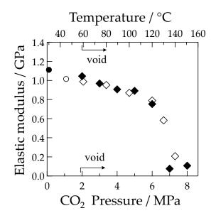
**Figure 4.** Elastic modulus of the OD-PC as a function of temperature and CO<sub>2</sub> pressure;  $\bigcirc$ , temperature;  $\bullet \blacklozenge$ , CO<sub>2</sub> pressure;  $\bigcirc \bullet$ , without void;  $\diamondsuit \blacklozenge$ , void.
