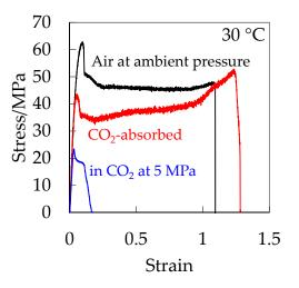
**Figure 12.** Stress–strain curve of OD-PC under air at atmospheric pressure in  $CO_2$  at 5 MPa and  $CO_2$ -absorbed PC under air at atmospheric pressure after absorbing and releasing  $CO_2$  of 5 MPa.
