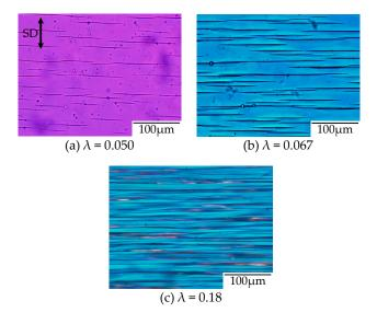
**Figure 9.** Polarized optical micrographs of OD-PC obtained by stretching under  $CO_2$  at 5 MPa at various strains.
