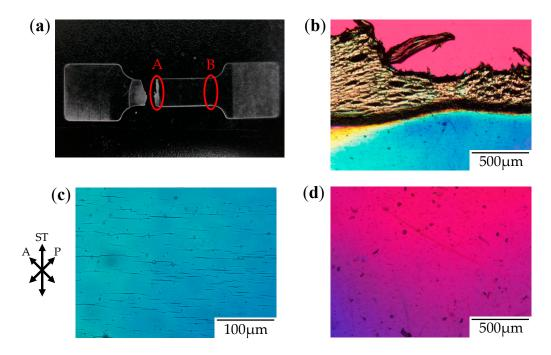
**Figure 3.** Photograph and polarized optical micrographs of OD-PC obtained by stretching under atmospheric pressure at 120 °C. (a) Photograph of the fractured specimen; (b) Polarized optical micrograph for region A; (c) Magnification of the lower part of (b); and (d) Polarized optical micrograph for region B.
