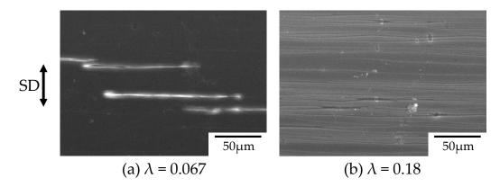
**Figure 10.** Scanning electron microscope (SEM) micrographs of the surface of the stretched OD-PC obtained by stretching under  $CO_2$  at 5 MPa at strains corresponding to Figure 9b,c.
