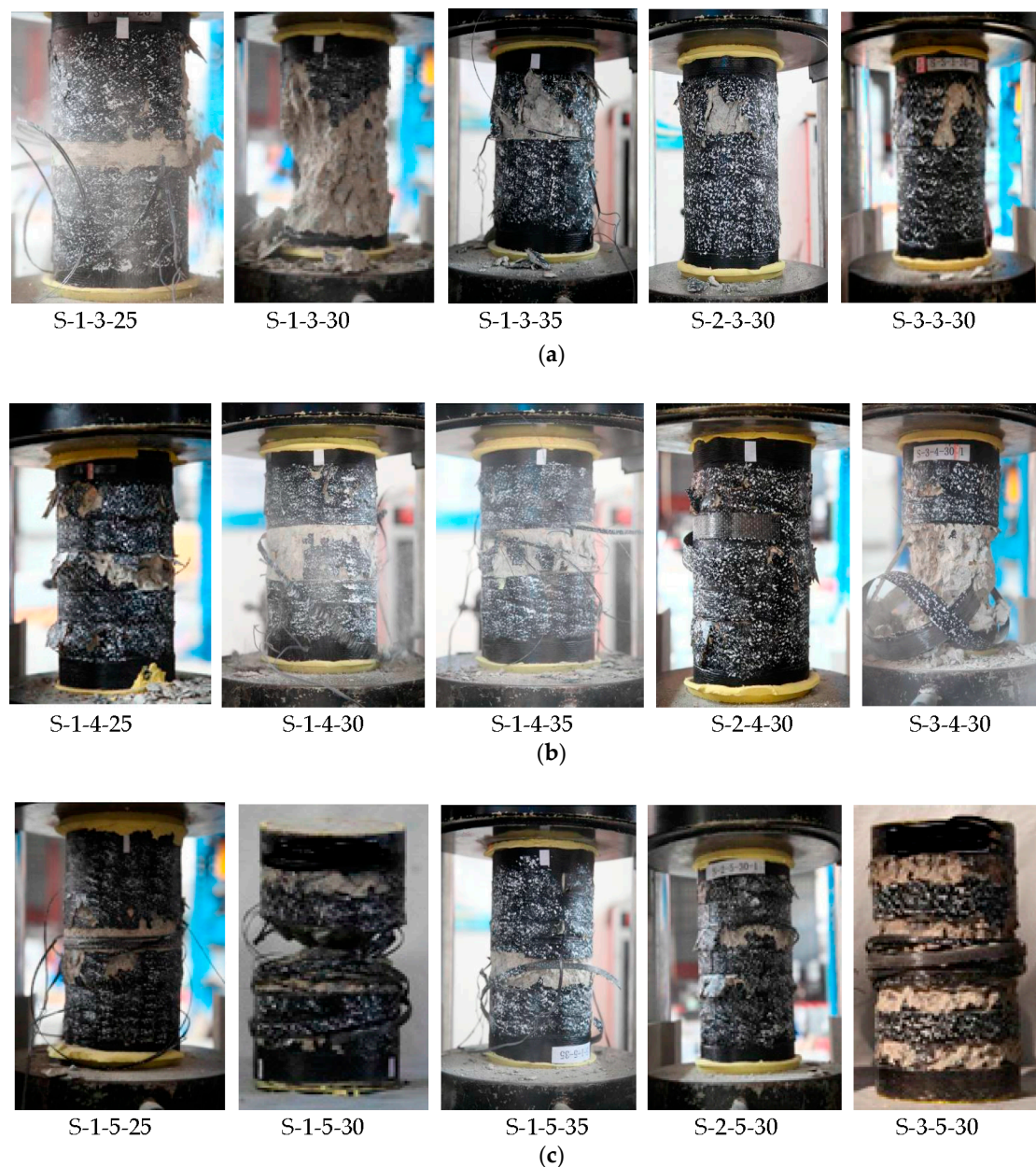
Figure 8. Failure modes. (a) Specimens wrapped with three FRP strips; (b) Specimens wrapped with four FRP strips; (c) Specimens wrapped with five FRP strips.
