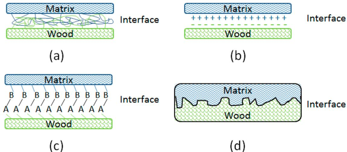
**Figure 7.** Wood-matrix interfacial bonding mechanisms: (a) molecular entanglement following interdiffusion, (b) electrostatic adhesion, (c) chemical bonding, and (d) mechanical interlocking.
