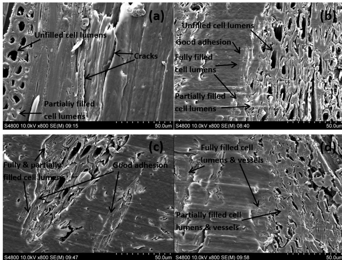
**Figure 6.** SEM photographs of cross section of untreated (a), MAPE treated (b), Si69 treated (c), and VTMS treated (d) composites.
