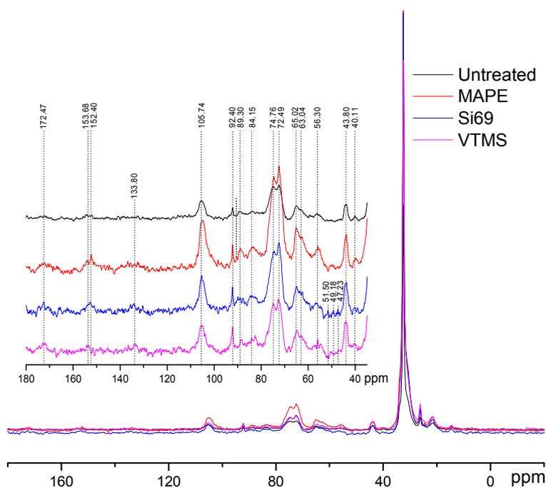
Figure 3.  $^{13}\text{C}$  NMR spectra of untreated, MAPE, Si69 and VTMS treated WPC.
