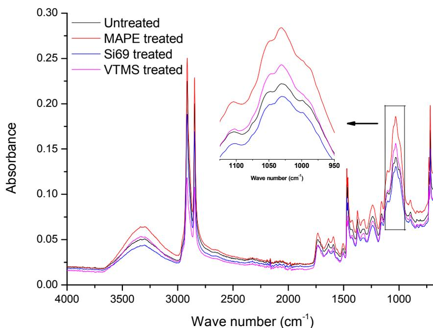
**Figure 1.** Fourier Transform Infrared spectroscopy (FTIR) spectra of untreated, maleated polyethylene (MAPE), bis(triethoxysilylpropyl)tetrasulfide (Si69), and vinyltrimethoxysilane (VTMS) treated wood plastic composites (WPC).
