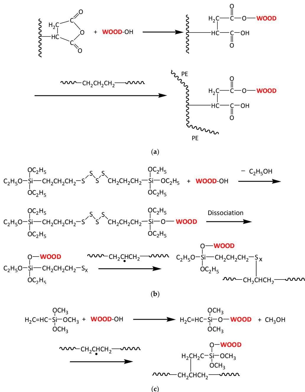
**Figure 2.** Proposed chemical reactions between the coupling agents ((a) MAPE; (b) Si69; (c) VTMS) and the raw materials of the composites.
