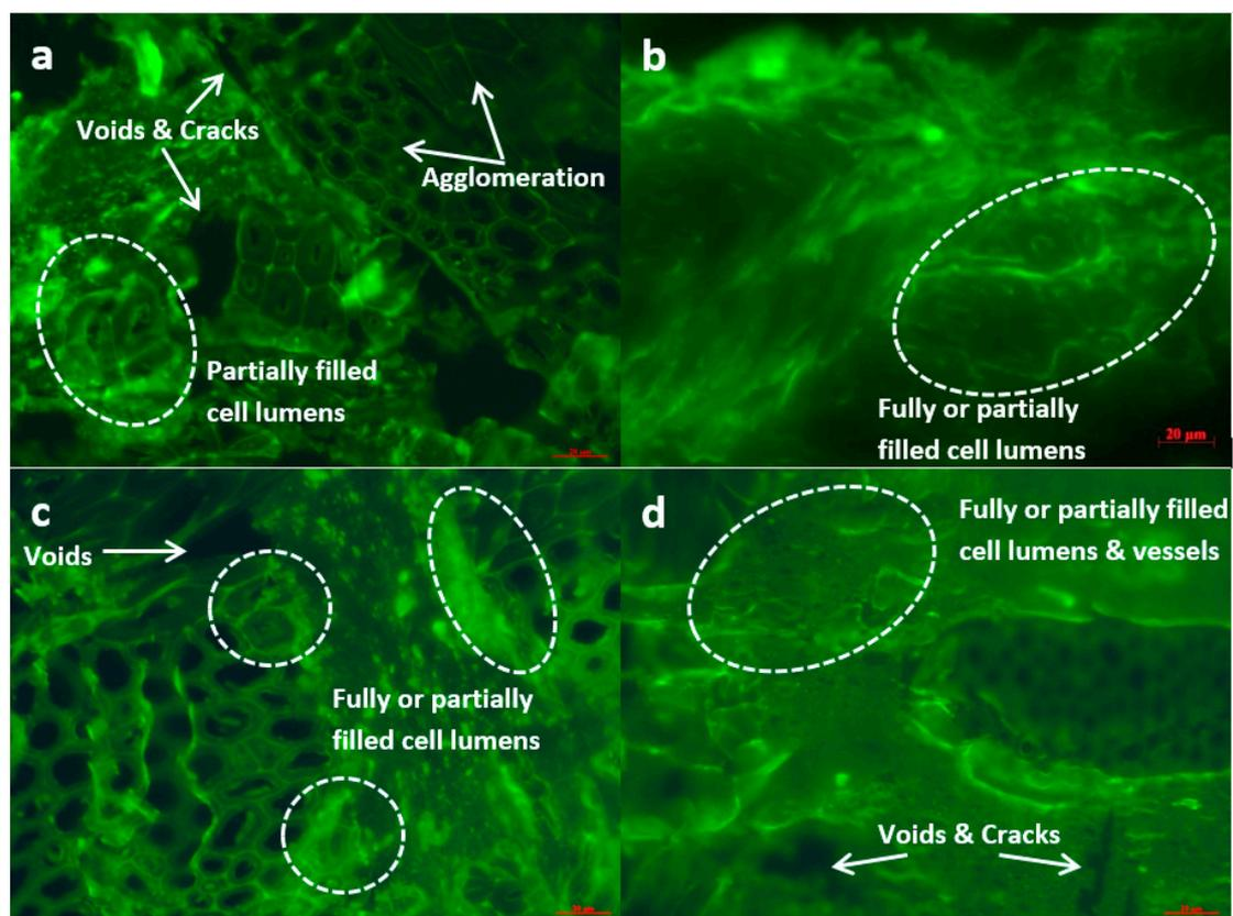
**Figure 5.** Fluorescence Microscope (FM) photographs of cross section of untreated (a), MAPE treated (b), Si69 treated (c), and VTMS treated (d) composites.
