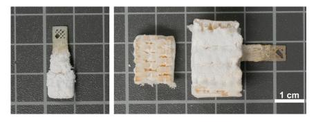
**Figure 5.** Mineral-coated samples: scaffold type P2 (sample G03 (**left**)) and scaffold type P3 (sample G07 (**center** and **right**)). Sample shown in the center is cut open to show the inner section of the scaffold. The scale bar applies to all images.
