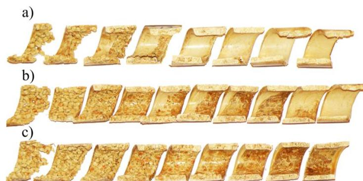
**Figure 4.** The effect of screw speed on the material flow in the screw channel (samples of the material of 40% WF content removed from the screw): (a)  $N = 20$  rpm, (b)  $N = 50$  rpm, (c)  $N = 80$  rpm.
