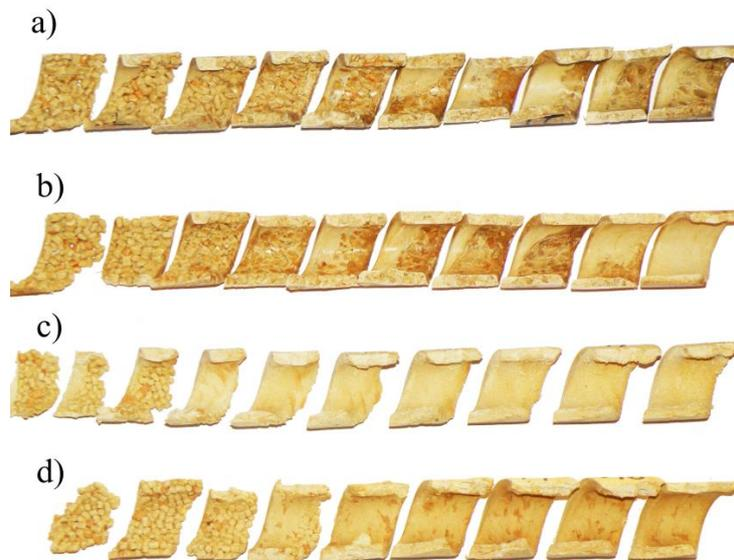
**Figure 3.** The effect of wood flour (WF) content on the material flow in the screw channel (samples of the material of different wood content removed from the screw, obtained by extrusion at the screw speed  $N = 50$  rpm): (a) WF = 30%, (b) WF = 40%, (c) WF = 50%, (d) WF = 60%.
