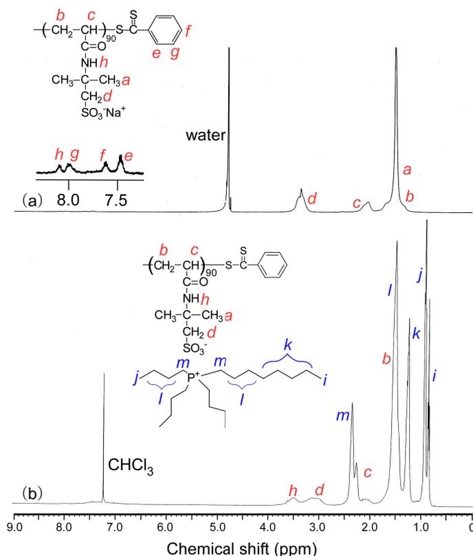
**Figure 2.**  $^1\text{H}$  NMR spectra for (a) PAMPSNa in  $\text{D}_2\text{O}$  and (b) PAMPSP $_{4448}$  in  $\text{CDCl}_3$ .
