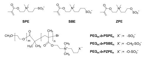
**Figure 1.** Structure of the zwitterionic monomers employed, and of the block copolymers synthesized and investigated. The number average degree of polymerization,  $DP_n$ , of the PEG block was kept constant as m = 114. For the  $DP_n$  values n of the various polyzwitterion blocks, see "Results and Discussion".
