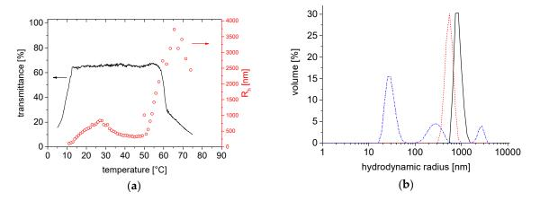
**Figure 7.** Temperature dependent study (cooling run) of 3.0 g·L<sup>-1</sup> solutions in NSS of ZPE-based block polymer PEG-*b*-PZPE-1: (**a**) by turbidimetry (cooling run); values for the apparent average hydrodynamic radius  $R_h$  are also shown (**O**); (**b**) distributions of the hydrodynamic radii at 11 °C (------), 35 °C (-----), and 75 °C (---).
