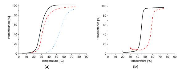
**Figure 4.** Temperature-dependent turbidity (cooling runs) of: (**a**) 30.0 g·L<sup>-1</sup> aqueous solutions of SPE-based block polymers PEG-*b*-PSPE-3 (—), PEG-*b*-PSPE-4 (- - -) and PEG-*b*-PSPE-5 (- - -); (**b**) 3.00 g·L<sup>-1</sup> solutions of PZPE homopolymers PZPE-1 (—) and PZPE-2 (- - -) in NSS.
