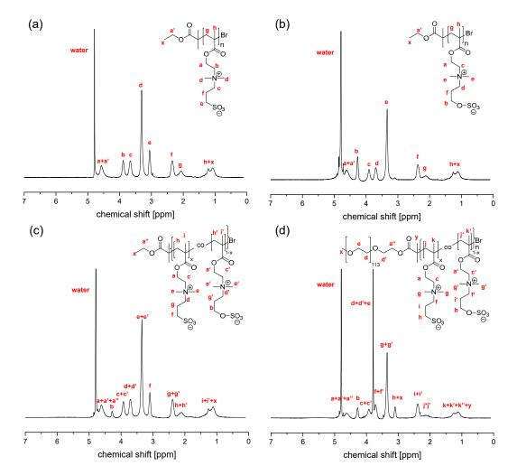
**Figure 3.** <sup>1</sup>H NMR spectra in 0.5 M aq NaCl (D<sub>2</sub>O) of (**a**) homopolymer PSPE-2, (**b**) homopolymer PZPE-1, (**c**) statistical copolymer P(SPE-*co*-ZPE)-1, and (**d**) statistical block copolymer mPEG-*b*-P(SPE-*co*-ZPE)-2.
