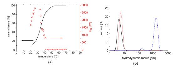
**Figure 8.** Temperature dependent study of 3.0 g·L<sup>-1</sup> solutions of statistical block copolymer PEG-*b*-P(SPE-*co*-ZPE)-2 in NSS: (**a**) by turbidimetry (cooling run); values for the apparent average hydrodynamic radius  $R_h$  are also shown. (**O**); (**b**) distributions of the hydrodynamic radii at 20 °C (------), 41 °C (-----), and 70 °C (---).
