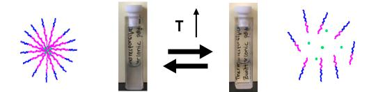
**Scheme 1.** Idealized view of the temperature-induced micellar assembly/disassembly of a thermoresponsive block copolymer induced by heating through an UCST-type transition, and the concomitant release of cargo molecules (•) that are solubilized inside of the micellar aggregate at elevated temperature.
