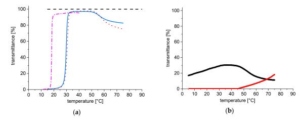
**Figure 5.** Temperature dependent turbidity of 30 g·L<sup>-1</sup> aqueous solutions of sulfobetaine polymers: (a) PSPE-1 (----), mPEG-Br (----), and 1:1 w/w mixture of PSPE-1 and mPEG-Br in cooling (—) or (----) heating runs; (b) cooling runs of block copolymers PEG-*b*-PSBE-1 (—) and PEG-*b*-PSBE-2 (—).
