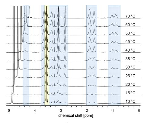
**Figure 6.** Temperature dependent <sup>1</sup>H NMR spectra of PEG-*b*-PSBE-1 in D<sub>2</sub>O.
