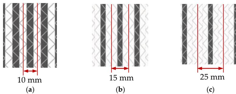
Figure 3. Schematics of sample cutting: (a) [C-G]; (b) [C-G-G]; (c) [C-G-G-G-G].
