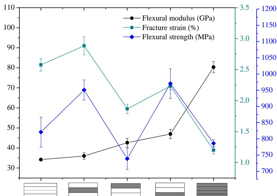
Figure 11. Flexural modulus, fracture strain, and strength of interlayer hybrid structure with C/G = 1:2.
