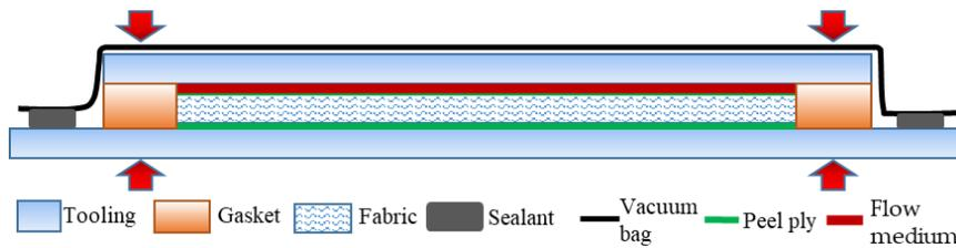
Figure 2. Schematic diagram of vacuum-assisted resin transfer molding (VARTM) process.
