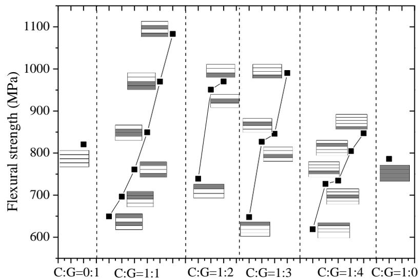
**Figure 15.** Flexural strength of interlayer hybrid structures with various stacking sequences and C/G hybrid ratios.
