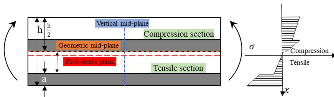
**Figure 8.** Stress distribution of a hybrid composite with low performance layers sandwiching high performance layers.
