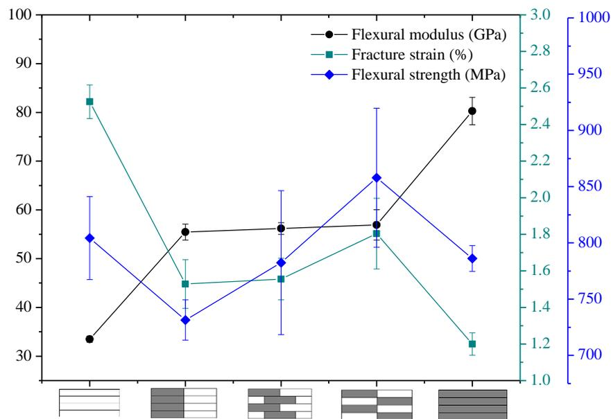
**Figure 16.** Flexural modulus, fracture strain, and strength of intralayer hybrid composite with various stacking sequences at C/G = 5 mm:5 mm.
