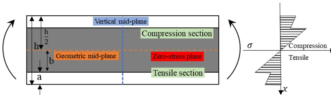
**Figure 9.** Stress distribution of an interlayer hybrid composite.
