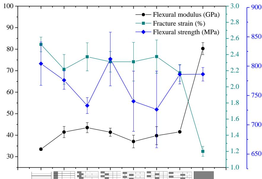
**Figure 18.** Flexural modulus, fracture strain, and strength of intralayer hybrid composite with various stacking sequences at C/G = 5 mm:20 mm.
