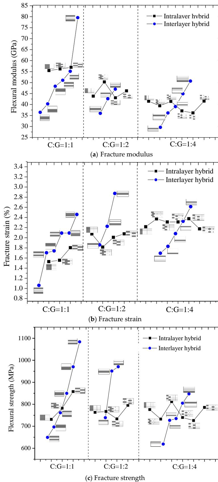
Figure 21. Flexural properties of interlayer and intralayer hybrid composites.
