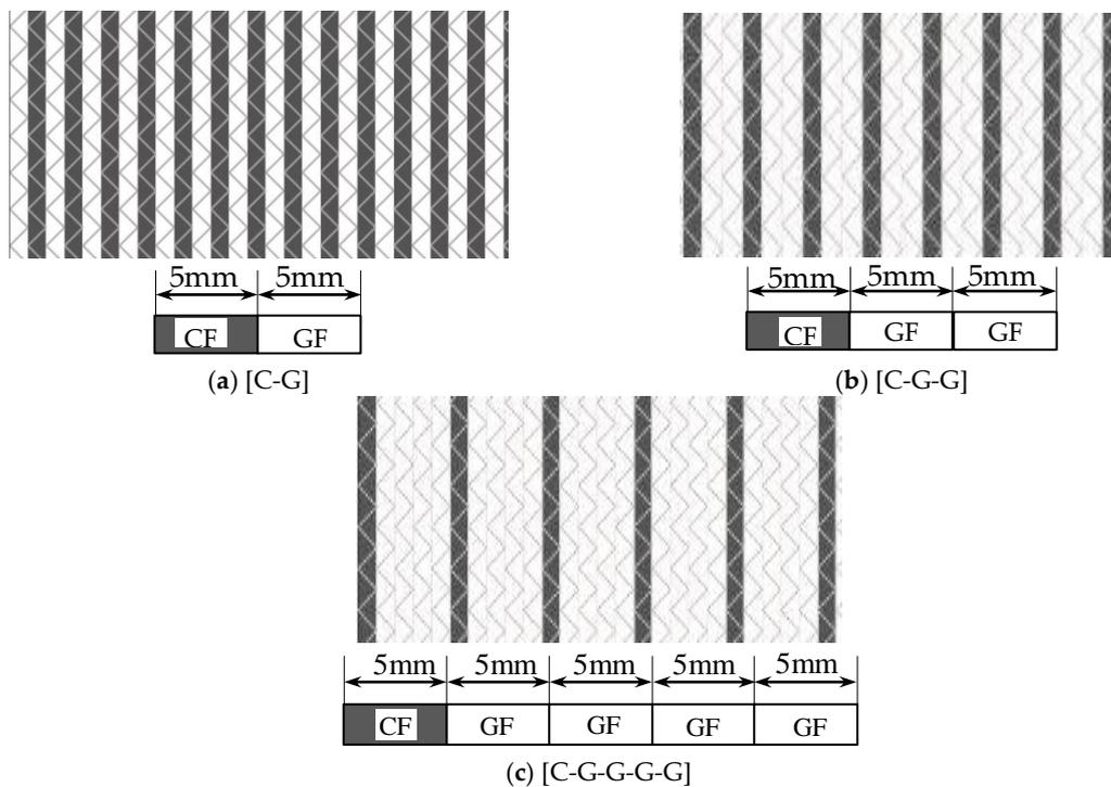
Figure 1. Schematic Structures of three types of non-crimp fabrics.
