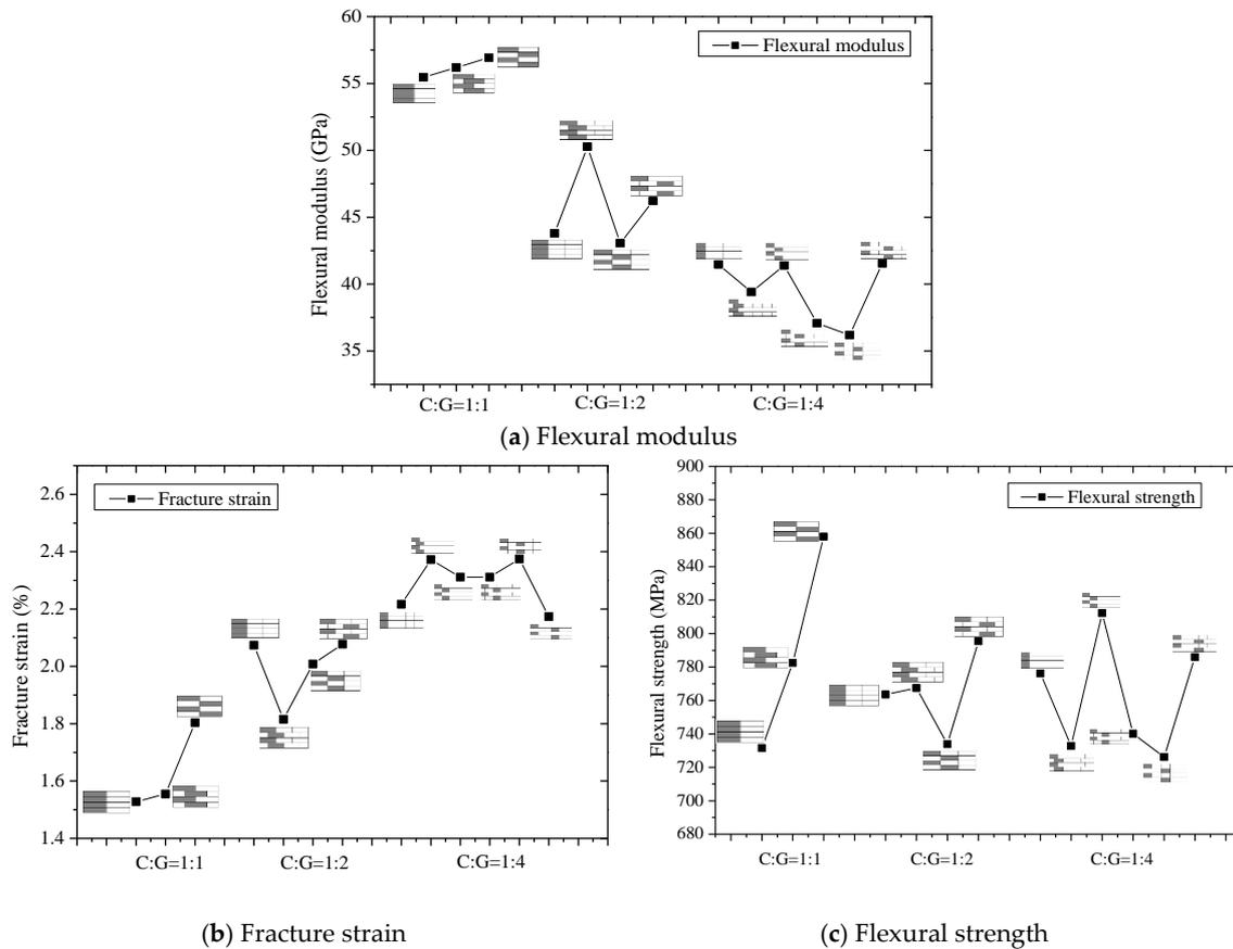
**Figure 19.** Flexural properties comparisons for various stacking sequences under three kinds of C/G ratios.
