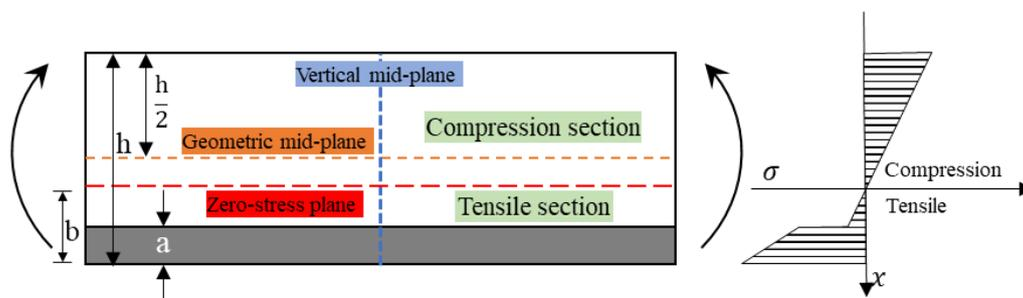
**Figure 6.** Bending stress distribution of an interlayer hybrid composite with high performance fiber distributed at the bottom surface.
