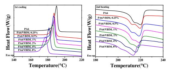
**Figure 3.** DSC first cooling (after 5 min isothermal for erasing heat history) and second heating curves of PA6 and the PA6/VBIM blends with different VBIM loadings.
