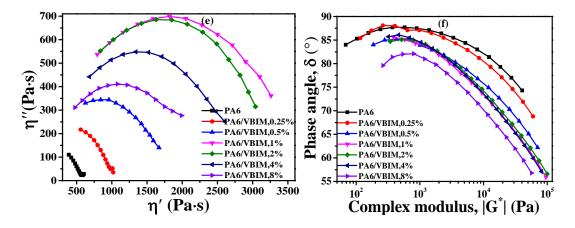
**Figure 6.** Linear viscoelastic properties from SAOS experiments: (**a**) storage modulus G'; (**b**) loss modulus G''; (**c**) complex viscosity  $|\eta^*|$ ; (**d**) damping factor tan  $\delta$  as functions of angular frequency; (**e**) Cole-Cole plots; and (**f**) vGP plots.
