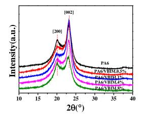
Figure 2. XRD patterns of neat PA6 and the PA6/VBIM blends.
