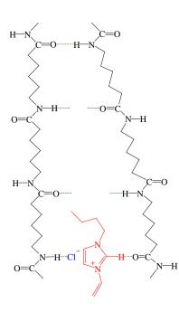
**Figure 12.** Schematic diagram of destruction and re-building of the hydrogen bond with the incorporation of excess VBIM.
