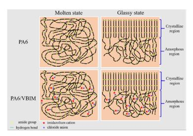
Figure 11. A schematic of the interactions between PA6 and VBIM under molten and glassy states.
