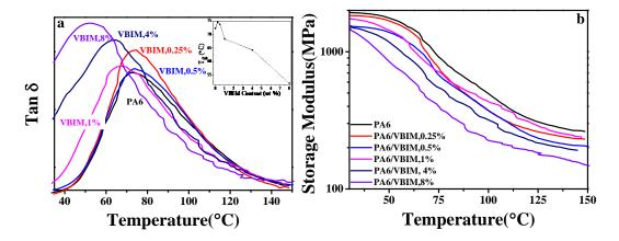
**Figure 4.** The loss tangent (**a**) and storage modulus (**b**) as functions of temperature for neat PA6 and the PA6/VBIM blends. The inserted sketch on the top right corner in Figure 4a shows how  $T_g$  varies according to VBIM contents in the blends.
