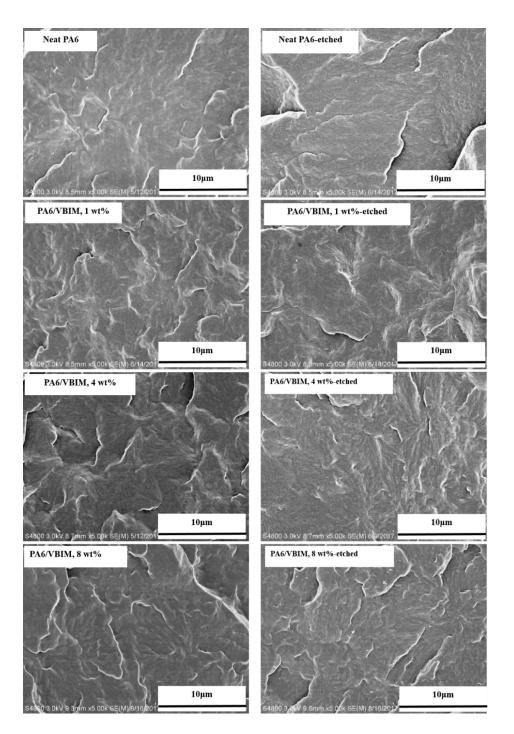
**Figure 1.** SEM images of the cross-fracture surface of PA6 and PA6/VBIM blends with different VBIM loadings before and after etching.
