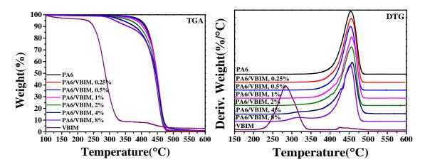
Figure 5. The TGA and DTG curves of neat PA6 and the PA6/VBIM blends.
