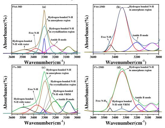
**Figure 10.** Curve-fitting of the N–H stretching band of (**a**) PA6 at room temperature; (**b**) PA6 at 250 °C; (**c**) PA6/VBIM, 1 wt % blend at room temperature; and (**d**) the PA6/VBIM, 1 wt % blend at 250 °C.
