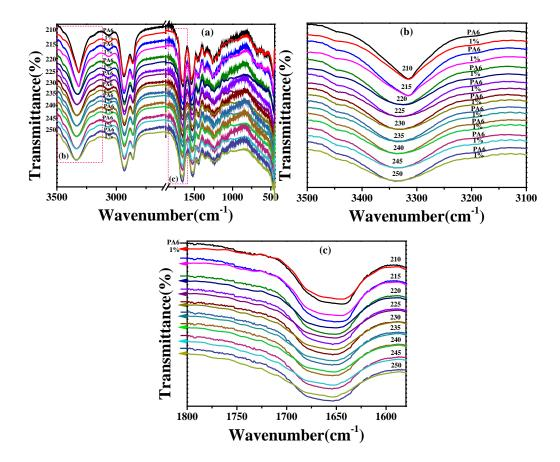
**Figure 9.** The temperature variable FTIR spectra from 210 to 250 °C of: (**a**) neat PA6 and the PA6/VBIM, 1 wt % blend; (**b**) zoomed area of the N–H stretching band; and (**c**) zoomed area of the amide I band.
