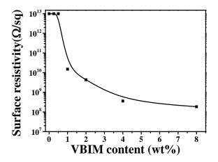
**Figure 8.** Surface resistivity of PA6 and the PA6/VBIM blends as a function of VBIM contents. This section may be divided by subheadings. It should provide a concise and precise description of the experimental results, their interpretation, as well as the experimental conclusions that can be drawn.
