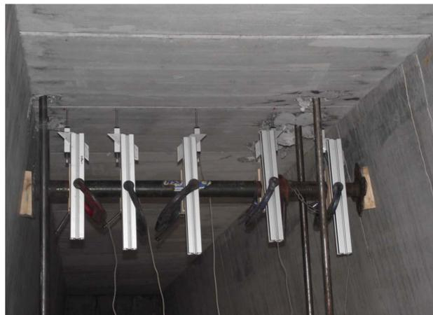
**Figure 4.** Position of the electronic displacement transducers.
