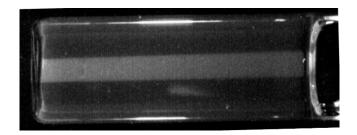
**Figure 8.** The image of a  $5 \times 5$  mm<sup>2</sup> 200 kVp X-ray beam propagating in a 60 mm length of RFG gel contained in a  $20 \times 20$  mm<sup>2</sup> cell. Optical artifacts occur at the glass/air sides of the cell and at the gel meniscus.
