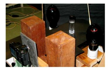
**Figure 14.** The set-up used to monitor, in situ, the fluorescence of an RFG gel on insertion of a seed of  $^{192}$ Ir. The main constituents are a  $20 \times 20 \text{ mm}^2$  glass cell containing the gel into which a 1.9 mm diameter catheter (shown in Figure 15) is inserted via a septum cap; two mercury-arc UV (365 nm) lamps, a Ricoh GX200 digital camera with a lead shield against gamma irradiation and wooden shields against direct UV.
