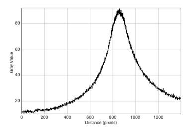
**Figure 16.** A pixel profile scan taken along the axis of the catheter, i.e., the centralvertical axis in Figure 15. The pixel resolution is 0.035 mm/pixel with a total scan length of approximately 50 mm.
