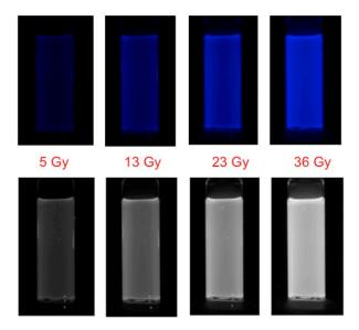
**Figure 2. Upper**: The full RGB color fluorescence in UV light of a  $10 \times 10 \text{ mm}^2$  cuvette containing a 1.4 mM solution of maleimido-pyrene in tertiary-butyl acrylate, as a function of accumulated dose in a GC200 γ-ray source (dose rate ~2 Gy/min). **Lower**: The same cuvette with the fluorescence shown as blue-pixel gray-scale values.
