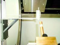
**Figure 9. Upper**: the PMMA RFG cell holder with a 20 mm thick RFG gel in a 50 mm diameter quarts cell for measurements in a "small animal" microbeam X-ray irradiation facility at the Antonie van Leeuwenhoek Ziekenhuis (Nederlands Cancer Institute) Amsterdam. **Lower**: a 6 mm gel positioned under the beam collimator, which could be rotated over 360 degrees in the X/Y plane.
