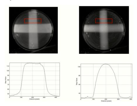
**Figure 11.** A 20 mm thick RFG gel irradiated with orthogonally-crossed X-ray beams. **Upper left**: a  $10 \times 10$  mm square beam, **Upper right**: a 10 mm diameter round beam. **Lower**: pixel profiles across the beams as shown by the red rectangles. Pixel resolution 0.049 mm/pixel.
