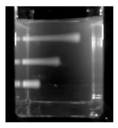
**Figure 13.** 80 MeV proton beam tracks imaged in a  $40 \times 40 \times 40 \text{ mm}^3$  RFG gel; attenuated, from top to bottom, by polystyrene sheets 22, 32, and 42 mm thick. Portal dose 15 Gy.
