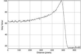
**Figure 12. Upper**: A grayscale image of an 80 MeV proton beam propagating in an RFG gel. **Lower**: A pixel-intensity profile along the axis of the beam; 0.061 mm per pixel.
