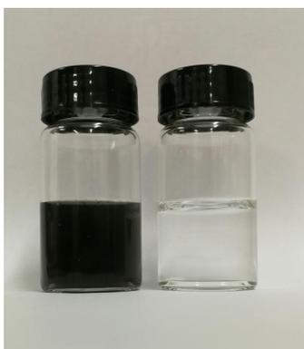
Figure 17. The feed (left) and permeating solution (right) obtained from M4.
