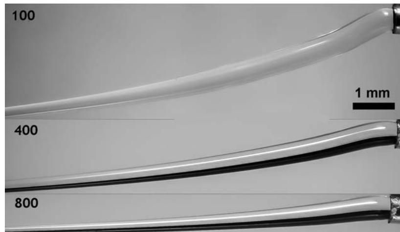
**Figure 10.** Extension of jets in PAN solution spinning at different rates (indicated in photos).
