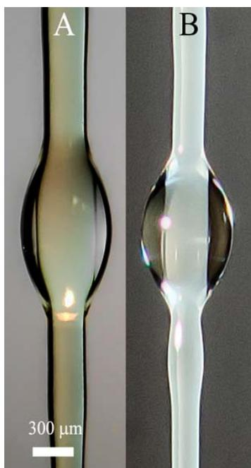
**Figure 8.** Enlarged images of solvent droplets on fiber surfaces for CPABI in DMAc solution (A) and PAN in DMSO solution (B).
