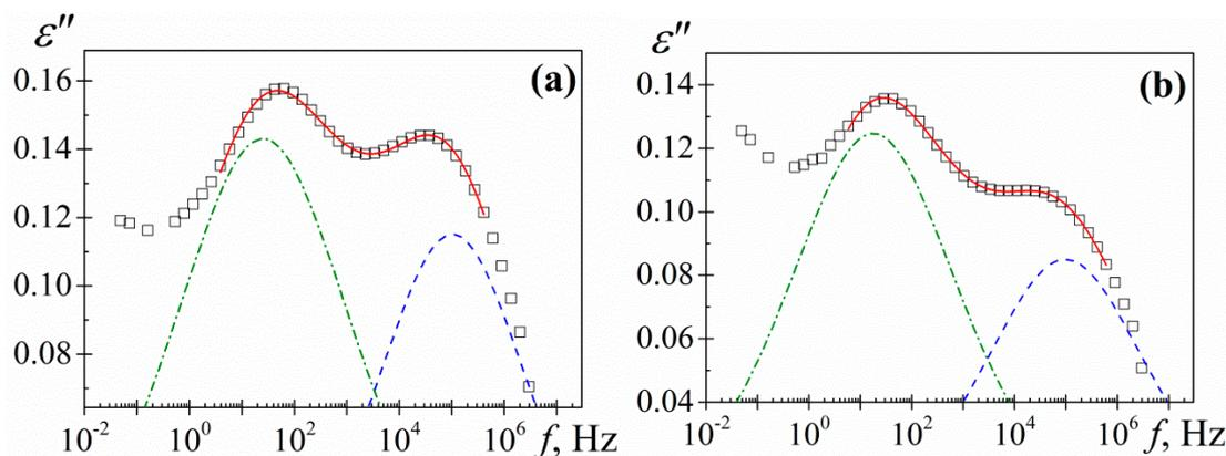
**Figure 10.** Deconvolution of loss factor for (a) PAzMa1 and (b) PAzMa2 at  $-70^\circ\text{C}$ . Squares represent the experimental data, continuous line the HN fitting curve and dashed lines the individual processes.
