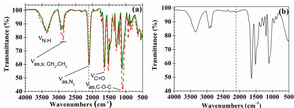
**Figure 3.** (a) Normalized ( $\nu_{as,N_3}$  peak) FTIR spectra of PAzMa1 (continuous line) and PAzMa2 (dash dot line) films and (b) FTIR spectra of PAzMa1 after thermal treatment (heated in TGA from rt to 250 °C at 1 °C·min<sup>-1</sup>).
