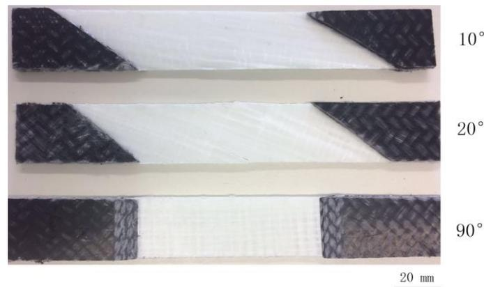
Figure 6. Macroscopic photographs of off-axis samples after the cyclic loading-unloading recovery test.
