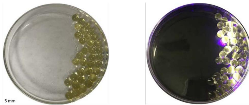
**Figure 5.** O-CDs embedded in sodium polyacrylate (SPA)-based beads under (left) regular light and (right) UV light.
