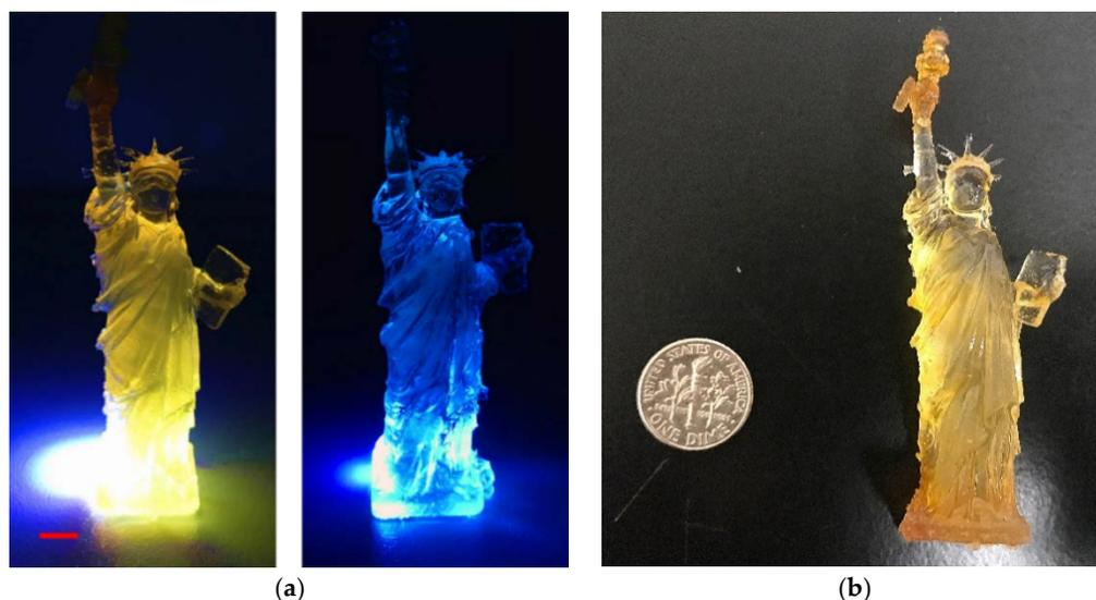
**Figure 8.** (a) 3D printing of the Statue of Liberty using (left) O-CDs and (right) control. (The bar is 5 cm); (b) The comparison of the specimen with a US dime.
