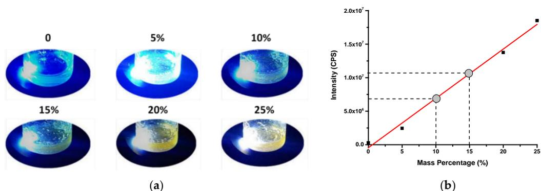
**Figure 7.** CDs-SPA mixed with the photopolymer resin with different mass percentage under UV lamp (365 nm) (a); The linear relation between the PL intensity (excitation: 425 nm; emission: 562 nm) and mass percentage of CDs-SPA in resin.  $R^2 = 0.99$  (b).
