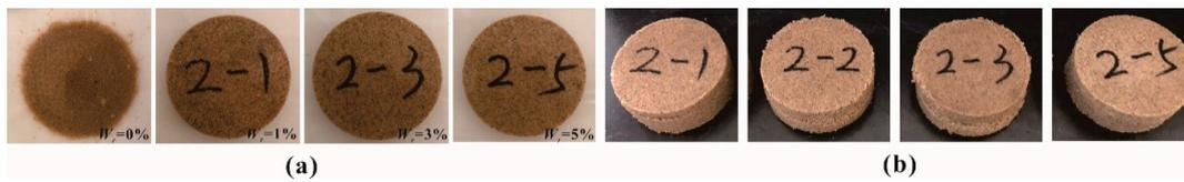
**Figure 4.** The shape of the polymer-sand composite material for different periods: (a) After immersion for 48 h; (b) After carrying out the direct shear test.
