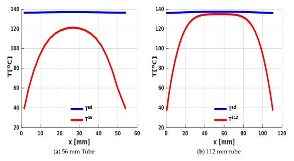
**Figure 7.** Adiabatic and nonadiabatic temperature profiles along an axis across the tubes (with maximum temperatures in the core) at a fixed time during the expansion process (**a**) in the 56 mm tube and (**b**) in the 112 mm tube.
