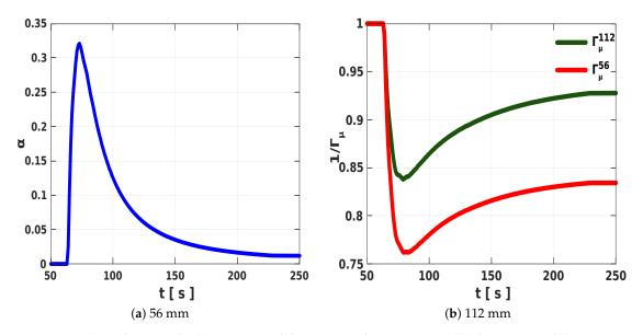
**Figure 8.** Plots showing the (**a**) variation of the computed  $\alpha$  in time and (**b**) the associated damping factor  $1/\Gamma_{\mu}$  in each tube as a consequence of thermal disparieties in the cylinders.
