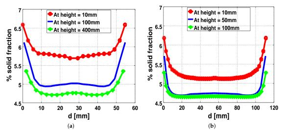
**Figure 10.** Simulation results showing the symmetric distribution of the solid foam fraction across the cylinder at different heights (**a**) in the 56 mm tube and (**b**) in the 112 mm tube.
