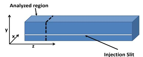
**Figure 1.** Schematic description of the geometry of the closed rectangular mold in the reaction injection molding (RIM) experiments. The marked region corresponds to the part of the expanded foam analyzed with  $\mu$ CT scans, (see Section 3.2).
