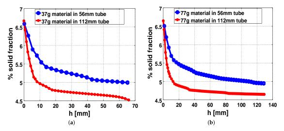
**Figure 11.** Disparity in foam-fraction distribution from the center of the base to a point in the core for both cylinders, with injected material mass of (**a**) 37 g and (**b**) 77 g.
