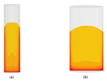
**Figure 9.** Spatial variation of solid foam fraction in the expanded foam (**a**) in the 56 mm diameter tube and (**b**) in the 112 mm diameter cylinder. The deep red region indicates higher solid fractions.
