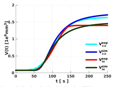
**Figure 5.** Fit functions for the volume data from the polyurethane (PU) foam-expansion experiments in the 112 mm with fit parameters values  $A_{112} = 1.7041$ ,  $\bar{\varepsilon}_{112} = 3.249,603$ ,  $\bar{\pi}_{112} = 3.293393$  and  $\gamma_{112} = 0.076$ , and the 56 mm tubes with parameter values  $A_{56} = 1.4288$ ,  $\bar{\varepsilon}_{56} = 3,049,603$ ,  $\bar{\pi}_{56} = 3.3$  and  $\gamma_{56} = 0.076$ .
