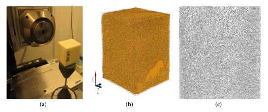
**Figure 3.** (a) Setup for the  $\mu$ CT scan data capture. (b) Reconstructed image of the  $\mu$ CT scan raw data using GeoDict. (c) Transversal binarised image of CT scan. Slice taken from middle point along the *z*-axis.
