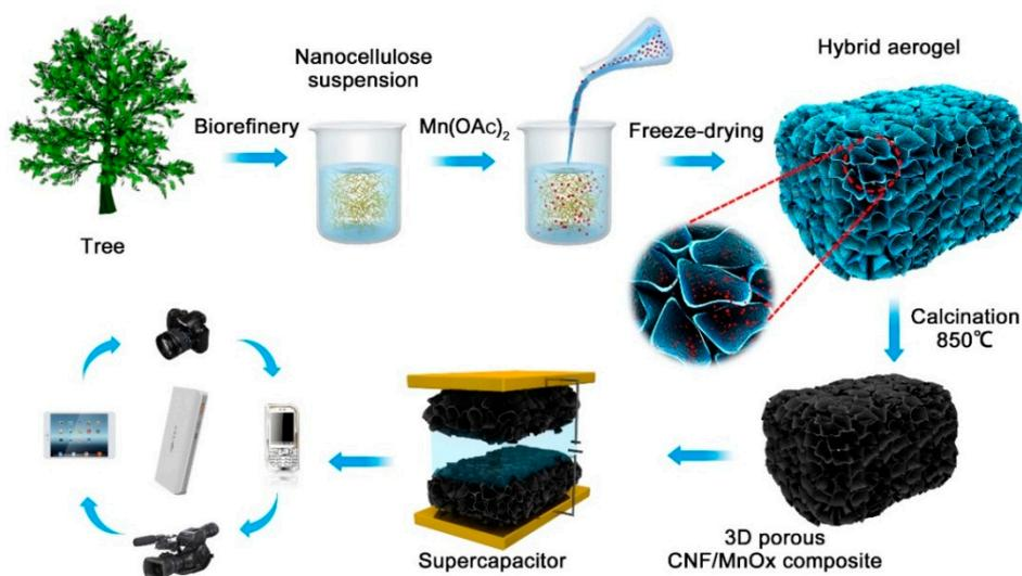
**Figure 1.** Schematic illustration of the preparation procedure of 3D porous carbonized nanocellulose fibers (CNF)/MnO<sub>x</sub> composite electrodes for supercapacitor applications.
