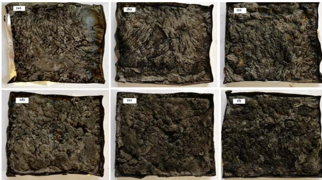
**Figure 6.** Photographs of the residues of PLA/APP10 (a), PLA/APP15 (b), PLA/APP20 (c), PLA/APP20/ST3 (d), PLA/APP20/ST5 (e), and PLA/APP20/ST7 (f) after cone calorimetry test.
