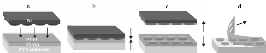
**Figure 1.** Schematic illustration of: (a) the assembly of poly(vinyl alcohol) (PVA) substrate film, a biodegradable PLGA device film, and a polytetrafluoroethylene (PTFE) film prior to the fabrication process; (b) hot punching is performed by applying pressure and heat; (c) a demolding step of the Ni stamp is completed, leading to separation of PLGA microcontainers from the surrounding film; (d) mechanical peeling of the surrounding PLGA film.
