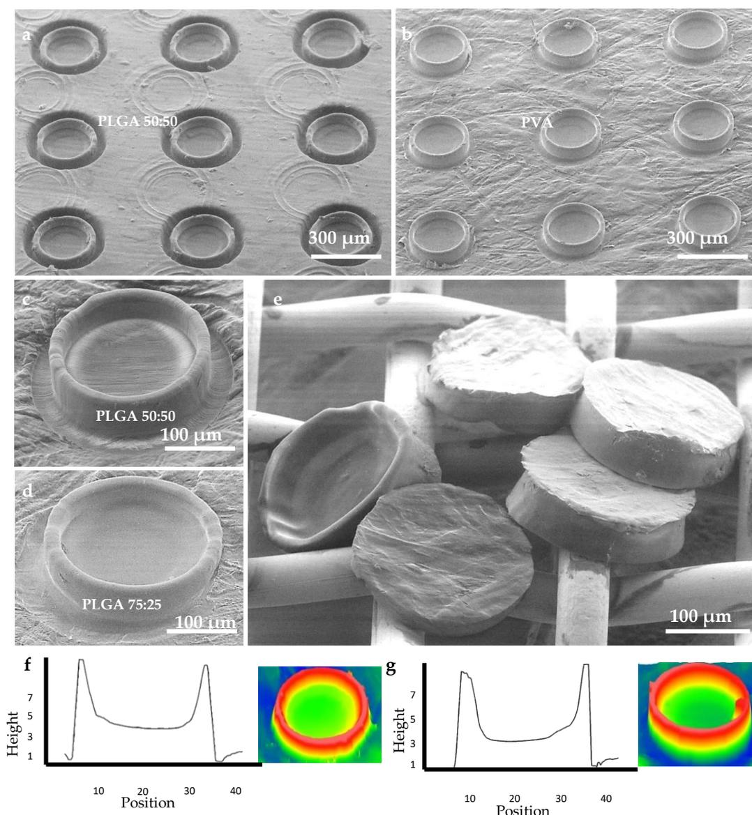
**Figure 2.** (a) SEM micrograph of microcontainer arrays before removal of the surrounding film; (b) microcontainer arrays after removal of the surrounding film; (c) close-up of a single PLGA 50:50 microcontainer; (d) close-up of a single PLGA 75:25 microcontainer; (e) harvested PLGA 50:50 microcontainers; (f) optical profile curve and 3D rendering of a single PLGA 50:50 microcontainer; (g) optical profile curve and 3D rendering of a single PLGA 75:25 microcontainer.
