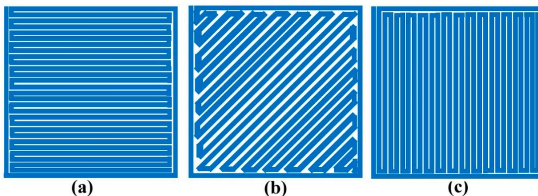
Figure S1 Design of 3D printed hydrogels with different infill angles (a) 0°, (b) 45° and (c) 90°.
