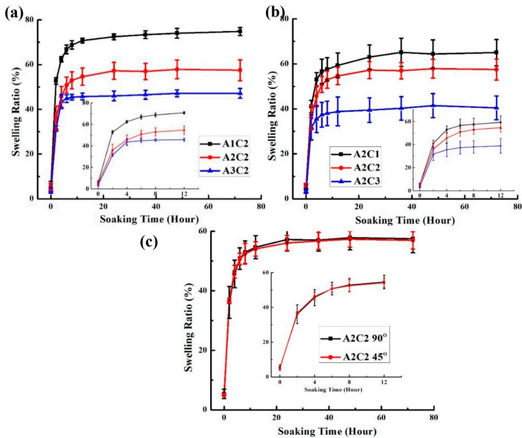
Figure S4 (a) swelling ratio of gel with different agar content, (b) swelling ratio of gel with different alginate content, and (c) Swelling ratio of A2C2 gel with different infill method.
