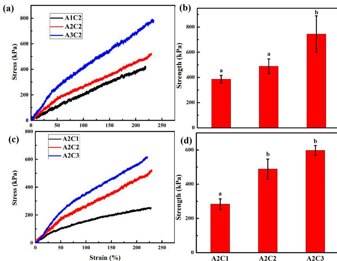
Figure S2, (a) Stress-Strain curve of 3D printed gel with different alginate concentration, (b) strength of 3D printed gels with different agar content ( $P > 0.05$ ), means with different letters are statistically different at  $P < 0.05$ , (c) Stress-strain curve of 3D printed gel with different agar concentration, and (d) strength of 3D printed gels with alginate content ( $P > 0.05$ ), means with different letters are statistically different at  $P < 0.05$
