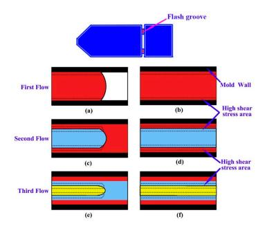
Figure S1. Schematic of multiflow vibrate-injection molding: (a, b) first flow; (c, d) second flow; and (e, f) third flow.
