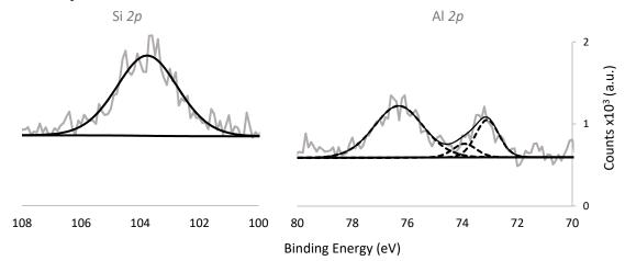
Figure 1: The fit and deconvolution of high-resolution Si 2p (left) and Al 2p (right) XPS spectra of 1% PTMS in aqueous solvent exposed to aluminium oxide for 5 seconds, obtained an Mg K $\alpha$  X-ray source.
