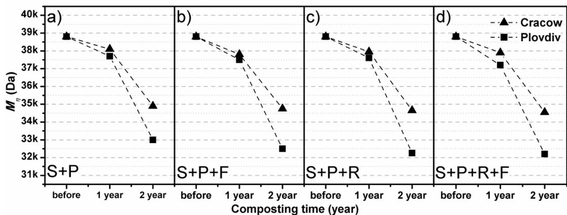
**Figure 2.** The changes in viscosity-average molecular weight of PLA during composting in: (a) soil with peat, (b) soil with peat covered with foil, (c) soil with peat and Radivit<sup>®</sup>, and (d) soil with peat and Radivit<sup>®</sup> covered with foil.
