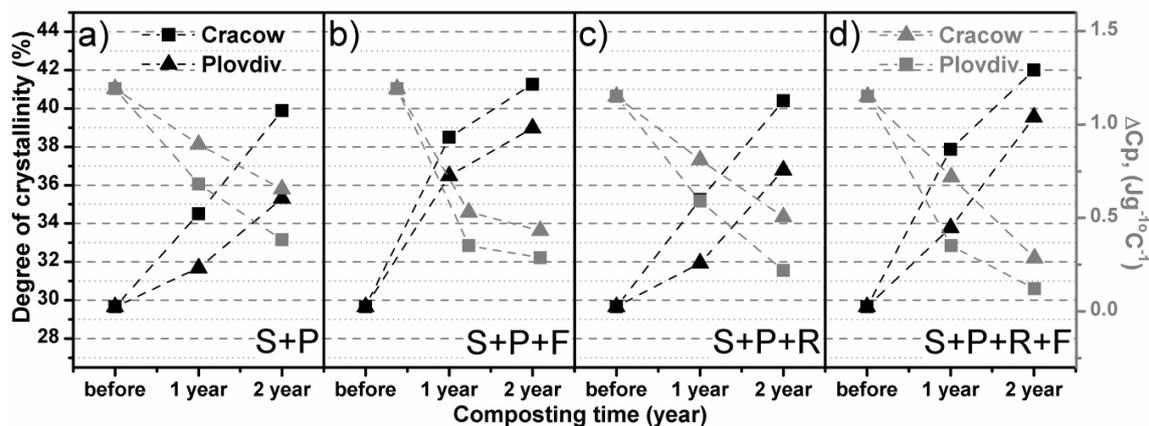
Figure 4. DSC analysis results of semicrystalline PLA spun-bonded mulching nonwovens before and after composting in: (a) soil with peat, (b) soil with peat covered with foil, (c) soil with peat and Radivit<sup>®</sup>, (d) soil with peat and Radivit<sup>®</sup> covered with foil.
