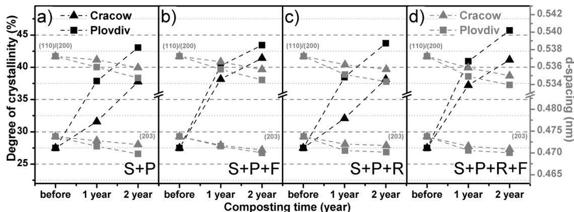
**Figure 6.** Numerical analysis results of WAXD diffractograms recorded for PLA spun-bonded mulching nonwovens before and after composting in: (a) soil with peat, (b) soil with peat covered with foil, (c) soil with peat and Radivit<sup>®</sup>, (d) soil with peat and Radivit<sup>®</sup> covered with foil.
