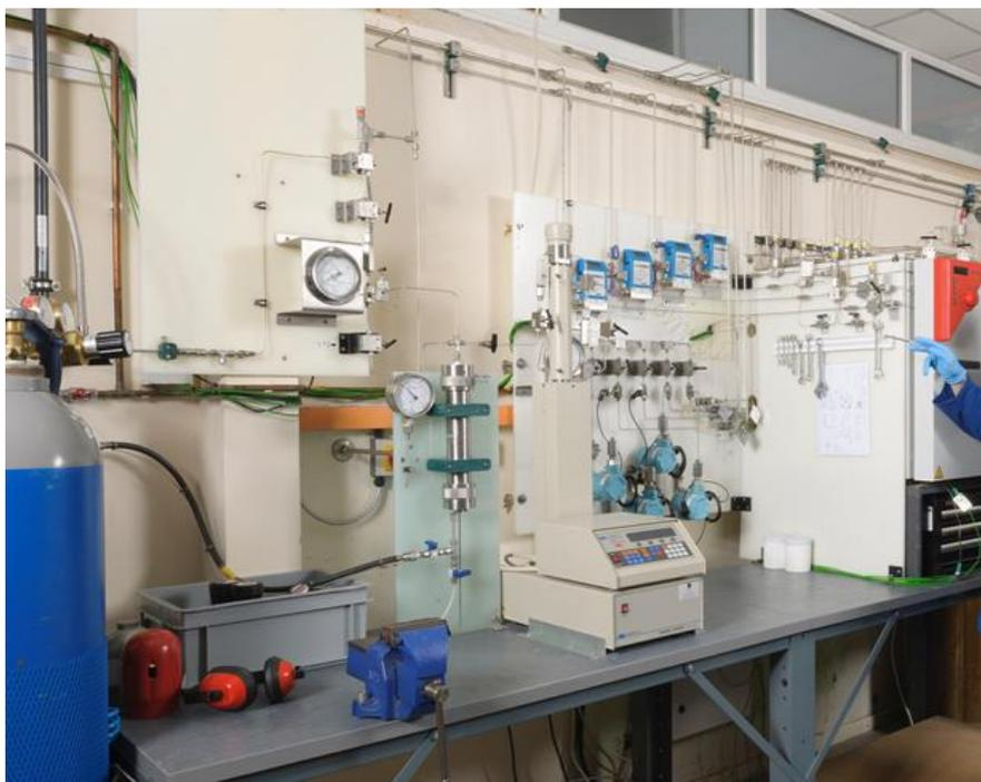
**Figure 1.** The custom-built rig used to expose polymers to supercritical CO<sub>2</sub> mixtures at pressures up to 689 barg.
