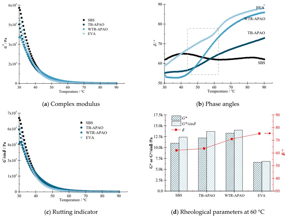
**Figure 1.** High-temperature rheological properties of asphalts via temperature sweep tests: (a) complex modulus, (b) phase angles, (c) rutting indicator, and (d) rheological parameters at 60 °C.
