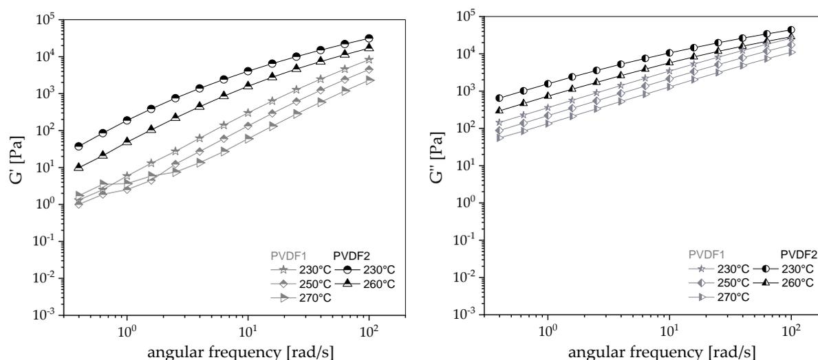
**Figure S1:** Storage modulus  $G'$  and loss modulus  $G''$  in dependence on the angular frequency of pure PVDF1 and PVDF2, measured at different temperatures.
