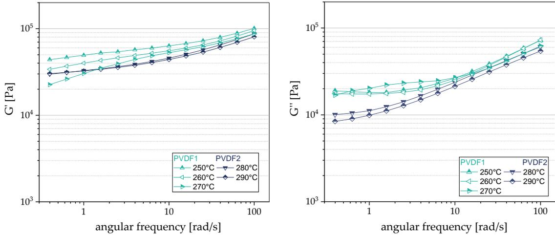
**Figure S2:** Storage modulus  $G'$  and loss modulus  $G''$  in dependence on the angular frequency of PVDF/1 wt% b-MWCNTs + 3 wt% CB composites, measured at different temperatures.
