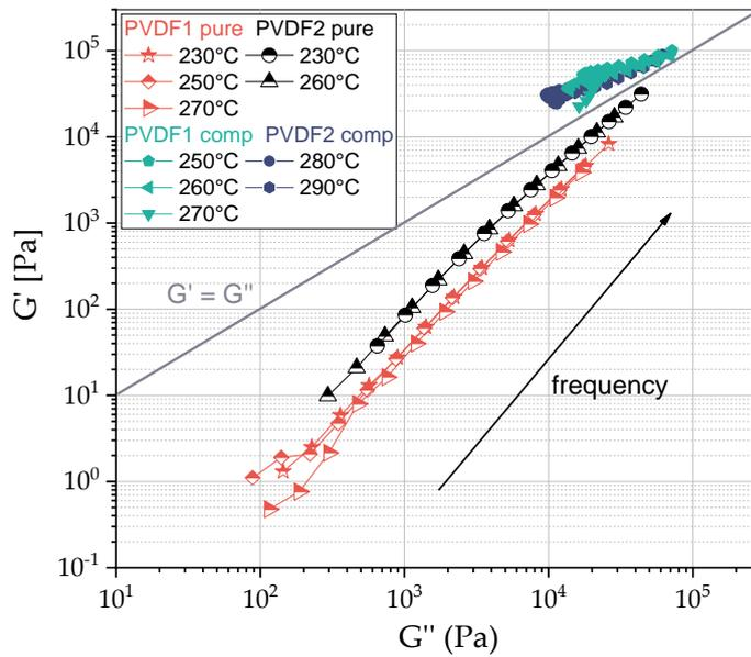
**Figure S3:** Storage modulus  $G'$  versus loss modulus  $G''$  from frequency sweeps as shown in Figs. S1 and S2 for pure PVDF1 and PVDF 2 and their composites with 1 wt% b-MWCNTs + 3 wt% CB, measured at different temperatures.
