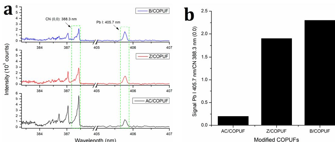
**Figure 7.** (a) LIBS spectra and (b) Pb I 405.7 nm/CN 388.3 nm (0,0) peak signal ratio of AC/COPUF, Z/COPUF, and B/COPUF after Pb<sup>2+</sup> adsorption, analyzed under high air pressure (760 Torr).
