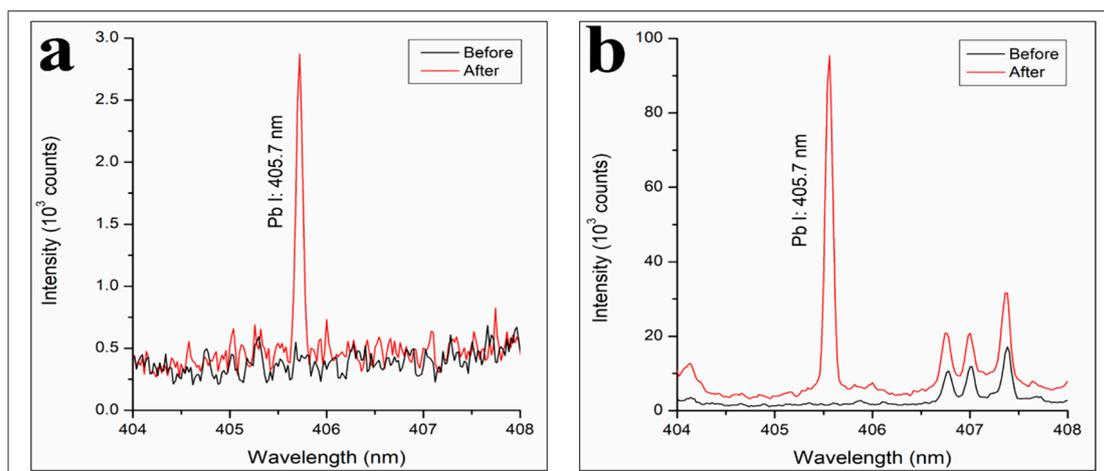
**Figure 8.** LIBS spectra of (a) COPUF and (b) B/COPUF before and after  $\text{Pb}^{2+}$  (100  $\mu\text{g}/\text{mL}$ ) adsorption, analyzed under low air pressure (3 Torr).
