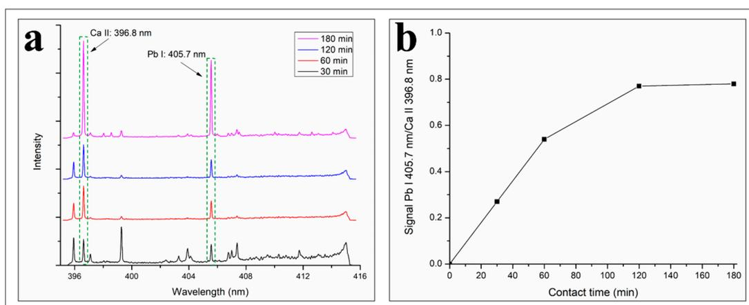
**Figure 9.** (a) LIBS spectra of B/COPUF after the adsorption of  $\text{Pb}^{2+}$  with a variation of contact time and (b) the Pb I/Ca II signal peak ratio.
