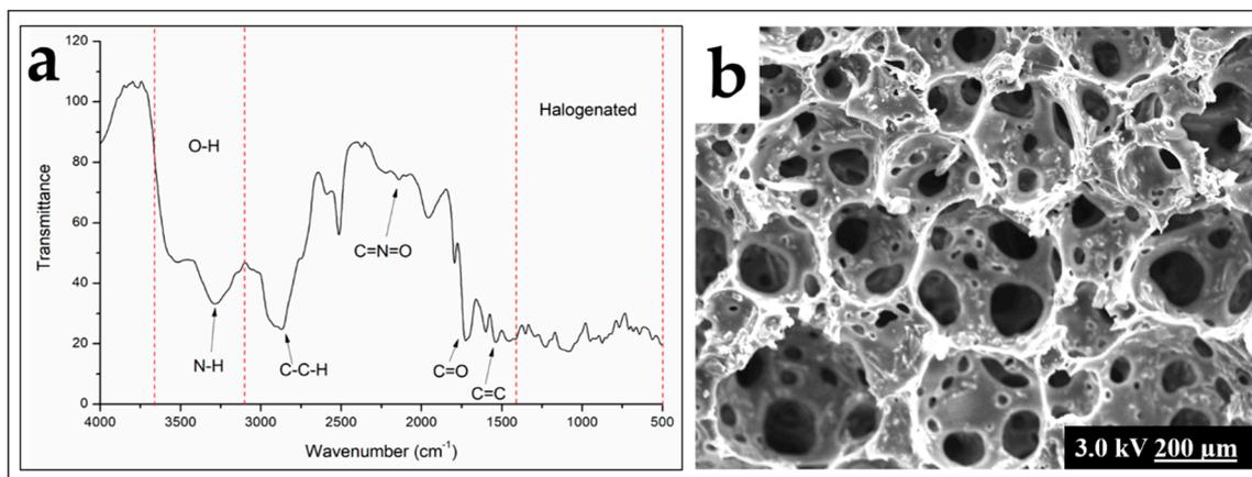
**Figure 12.** (a) Functional groups and (b) morphology characteristics of commercial PUF respectively analyzed with FTIR and SEM (200× magnification).
