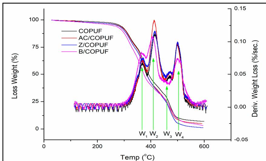
**Figure 6.** TGA and DTGA of COPUF, AC/COPUF, Z/COPUF, and B/COPUF with four stages of thermal degradation indicated by  $W_{1-4}$ .
