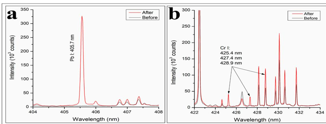
**Figure 11.** LIBS spectra of commercial PUF after and before the adsorption of (a)  $Pb^{2+}$  and (b) Cr (VI), analyzed at 83 mJ energy and 3 Torr air pressure.
