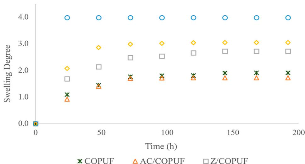
**Figure 5.** Swelling degree profile of COPUF, AC/COPUF, Z/COPUF, B/COPUF, and commercial PUF (CPUF).
