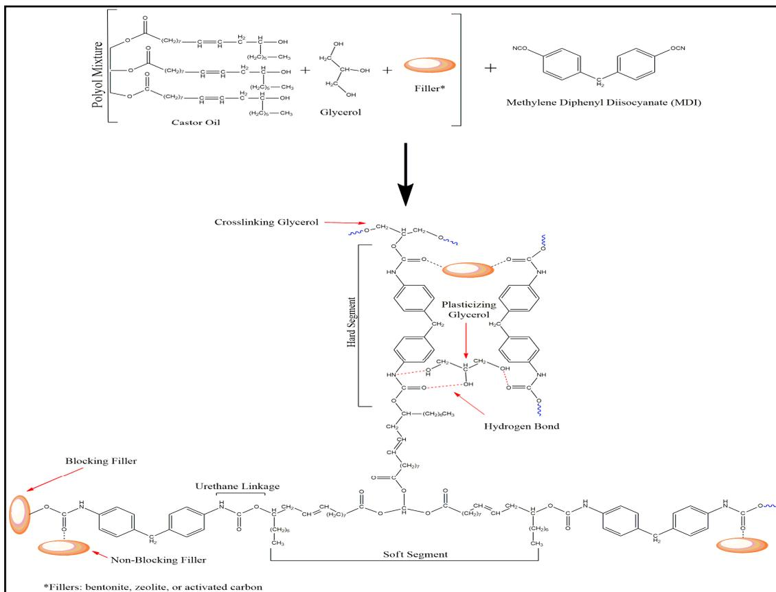
**Figure 1.** The reaction of castor oil-based PUF via the one-shot method with the addition of glycerol and fillers.
