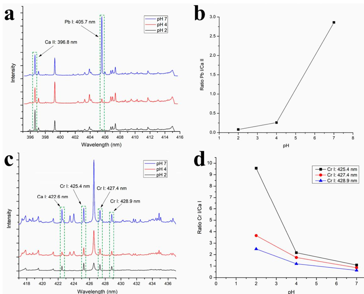
**Figure 10.** (a) LIBS spectra of B/COPUF and (b) the Pb I/Ca II signal peak ratio after the adsorption of  $Pb^{2+}$  (100  $\mu\text{g/mL}$ ) and (c) LIBS spectra of B/COPUF and (d) the Cr I/Ca I signal peak ratio after the adsorption of Cr (VI) (100  $\mu\text{g/mL}$ ).
