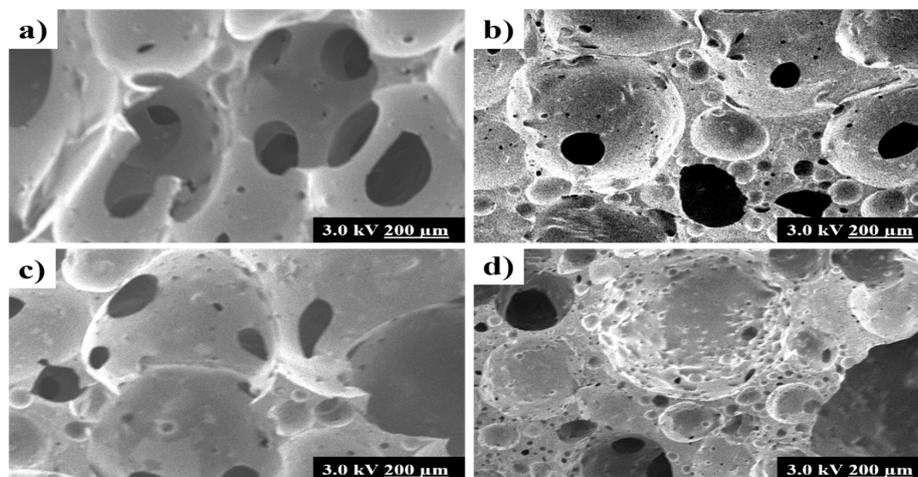
Figure 4. SEM images of (a) COPUF, (b) Z/COPUF, (c) B/COPUF, and (d) AC/COPUF.
