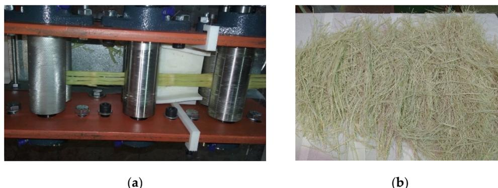
**Figure 2.** Fibre obtaining: (a) Stem passing through rolling mill device and (b) fibre bundles.
