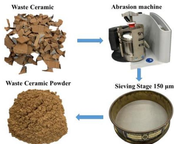
Figure 1. The preparation process of waste ceramic powder (WCP) in the laboratory.
