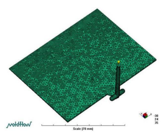
Figure 3. 3D-mesh on Moldflow analysis.
