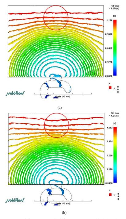
**Figure 6.** Melt front situation for different injection speeds. (a) Melt front uniformity. Mold temp:  $60 \degree C$ , Melt temp:  $245 \degree C$ , Injection speed  $10 \mbox{ cm/s}$ . (b) Melt front hysteresis. Mold temp:  $60 \degree C$ , Melt temp:  $245 \degree C$ , Injection speed  $3 \mbox{ cm/s}$ .
