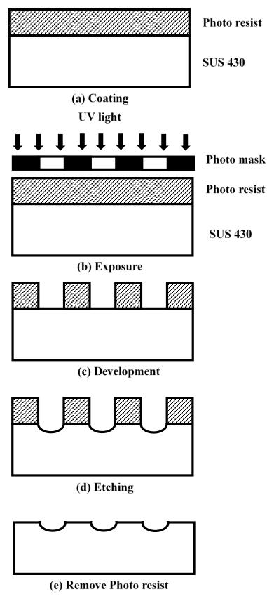
Figure 2. Process chart for photo-etching of mold insert.
