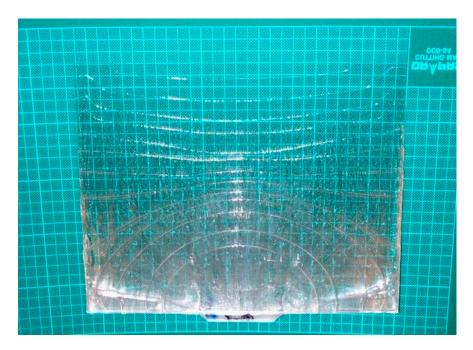
Figure 4. The bad flow situation of light guiding plate on micro-injection molding.
