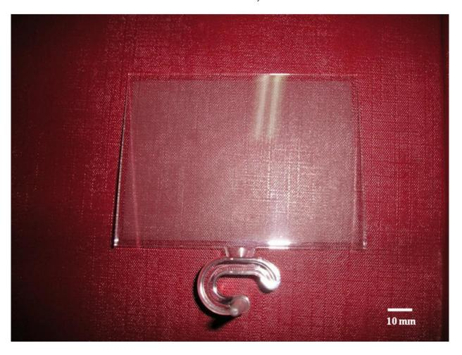
Figure 9. The molded light guiding plate.
