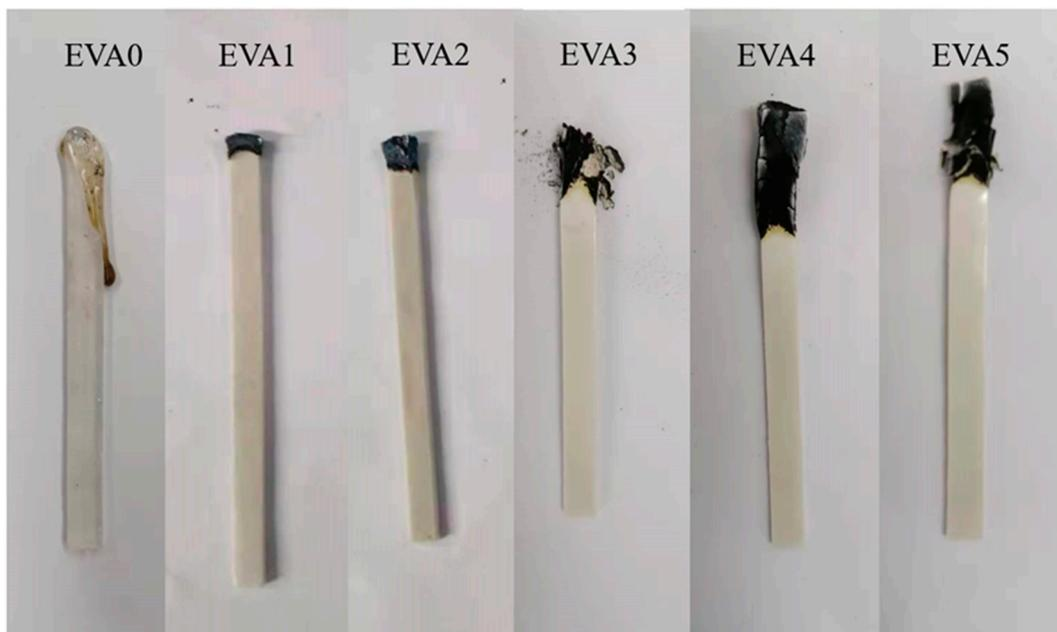
**Figure 7.** Digital photos of neat EVA and EVA/MH composites after LOI test.
