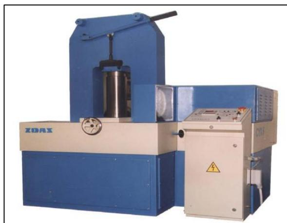
**Figure 1.** CYX 6/103 high-pressure isostatic press made by Žďas joint-stock company with a chamber volume of 2 L.
