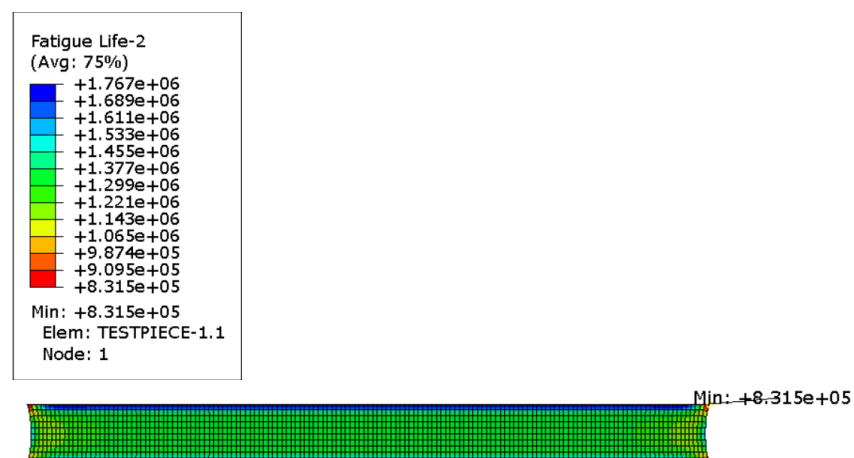
Figure 25. Life nephogram of plane tensile specimen.
