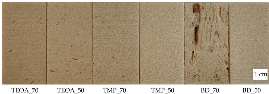
**Figure 4.** Rigid PUR foam samples' visual appearance.
