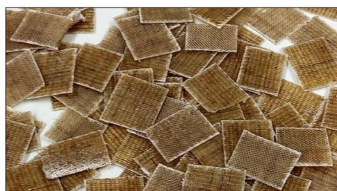
**Figure 3.** An example of a cut flax-fiber-reinforced epoxy composite with epoxide treatment and caffeine (1%).
