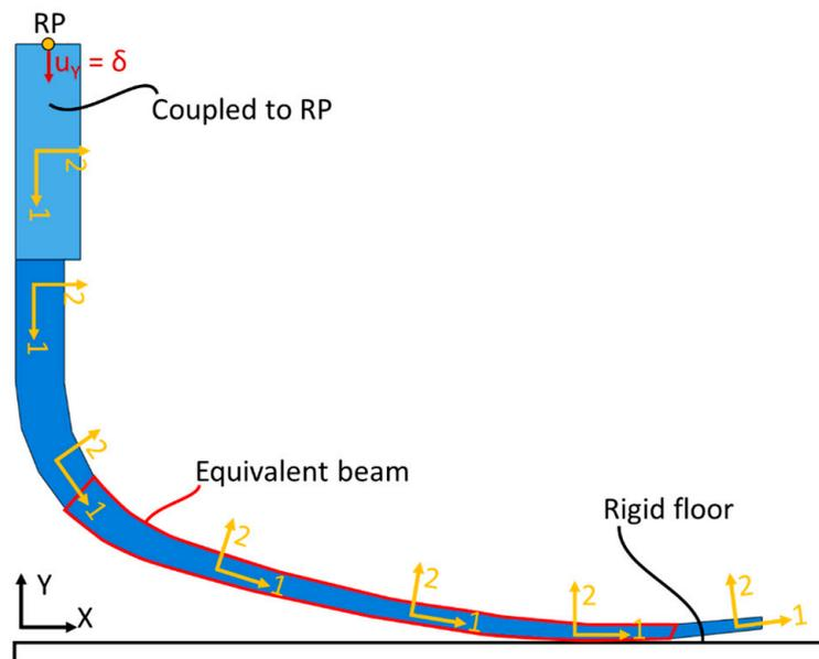
Figure 8. Model of the reference component.
