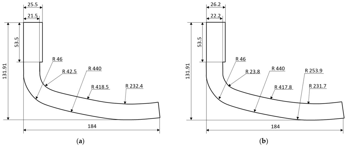
Figure 11. Optimised geometry of the prosthesis component considering a (a) T45 and a (b) R20 core.
