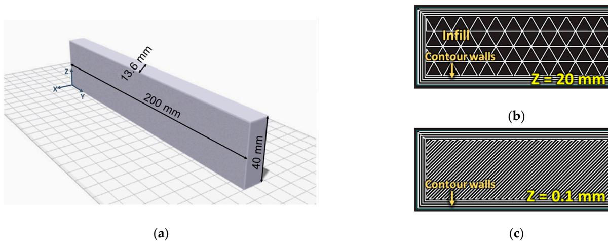
**Figure 1.** (a) 3PB specimen on a printing bed, (b) Central layers (with a triangular infill) and (c) Top/bottom layers.
