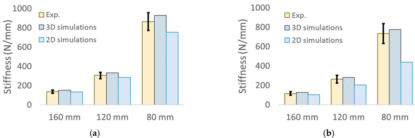
**Figure 9.** Stiffness results for the (a) T45 and the (b) R20 specimens.
