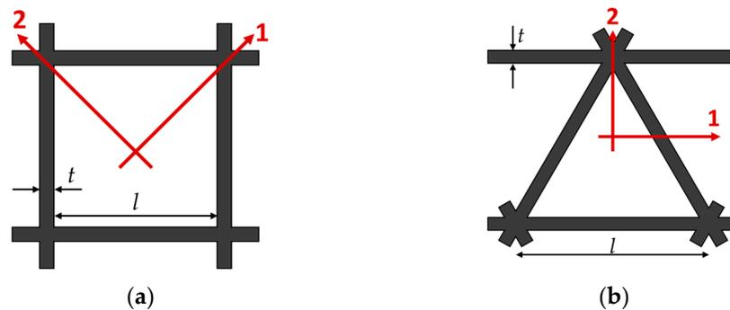
**Figure 6.** Core geometries for the analytical evaluations: (a) Rectangular and (b) Triangular.
