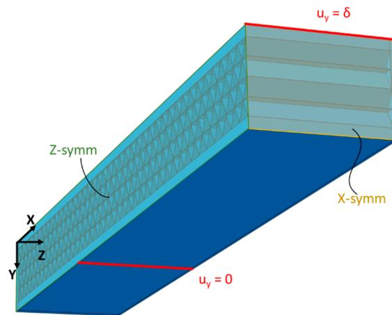
**Figure 5.** Three-dimensional 3PB simulation for the T45 core with a 160 mm span length.  $\delta$  refers to the applied displacement reported in Table 2 for the different simulations.
