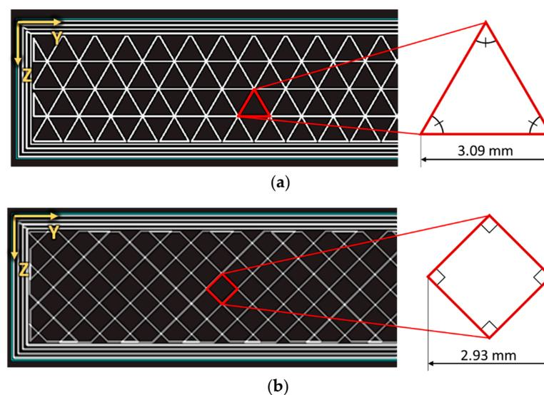
**Figure 2.** Extracted geometries of the unit-cells for the (a) T45 infill and the (b) R20 infill. Note that the for the R20 infill, the printer prints the infill with unidirectional layers (+45° or −45°); therefore, the figure (b) was obtained as the superposition of two subsequent layers.
