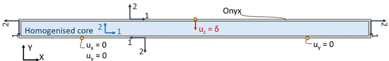
**Figure 4.** Two-dimensional 3PB simulations with a 160 mm span length. Axes 1–2 indicate local orientation.
