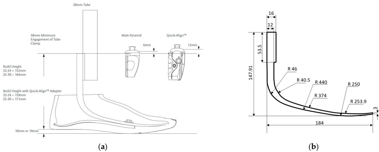
Figure 7. (a) The Össur VARI-FLEX™ design taken from [32] and (b) the inspired laminated component.
