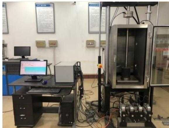
**Figure 2.** Uniaxial penetration test device.
