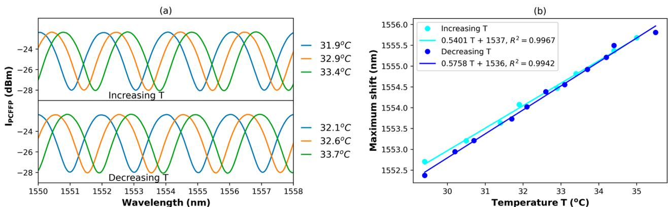
**Figure 3.** (a) Spectra of the measured  $I_{PCFPI}$  and (b) the characteristic curve of the wavelength shift for a PCFPI with a PDMS cavity in a range of temperature of 30 to 36 °C.
