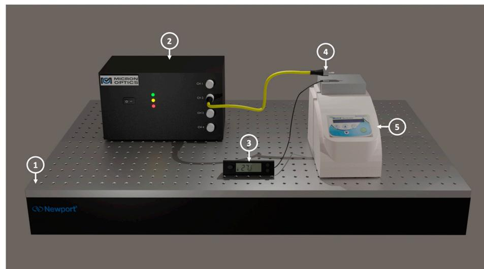
**Figure 2.** Experimental set-up used for temperature characterization: (1) optical table; (2) the sm125 interrogator; (3) digital thermometer with thermocouple; (4) ferrule connector with a polymer cap; (5) dry bath with block.
