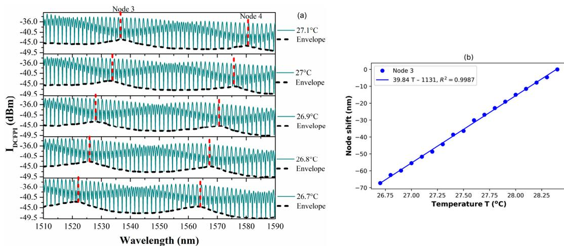
Figure 10. (a) Measured spectra of the DCFPI and (b) the characteristic curve of the node wavelength shift in the temperature range of 26.7 to 28.4 °C.
