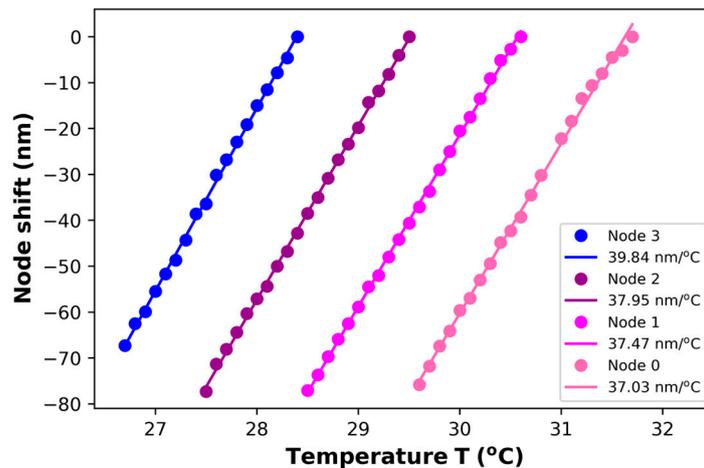
**Figure 11.** Characteristic curves of the wavelength shift of 4 nodes for a DCFPI using PDMS in a range of temperature of 26.7 to 31.7 °C.
