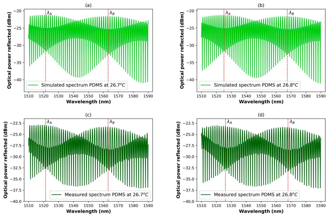
**Figure 4.** (a,b) Simulated and (c,d) experimental reflection spectra of a DCFPI when the surrounding temperature was  $26.7^\circ\text{C}$  and  $26.8^\circ\text{C}$ , respectively.
