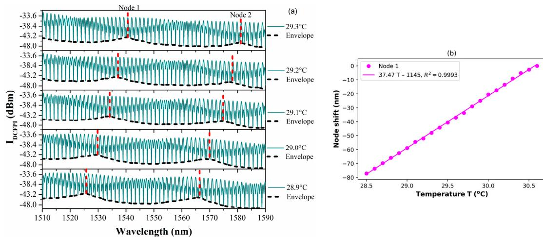
Figure 8. (a) Measured spectra of the DCFPI and (b) the characteristic curve of the node wavelength shift in the temperature range of 28.5 to 30.6 °C.
