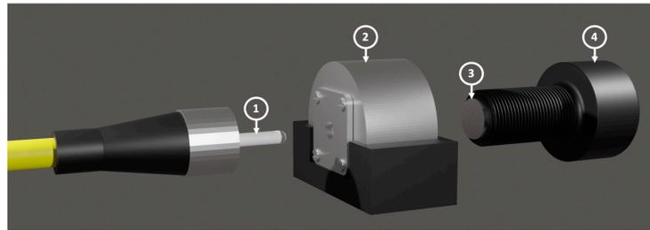
**Figure 5.** Components of the DCFPI sensor head: (1) Ferrule connector with a polymer cap; (2) Aluminum mount; (3) Plane mirror with a circular shape; (4) Fine thread screw.
