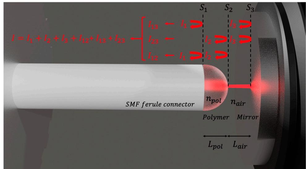
**Figure 1.** Internal view of the structure of the DCFPI-based temperature sensor.
