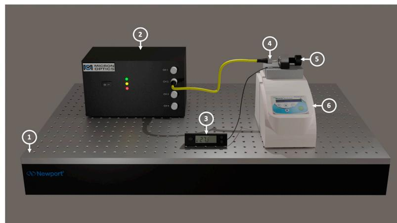
**Figure 6.** Experimental set-up used for temperature characterization of the DCFPI: (1) optical table; (2) the sm125 interrogator; (3) digital thermometer with thermocouple; (4) ferrule connector with a polymer cap; (5) screw with a mirror attached; (6) dry bath with block.
