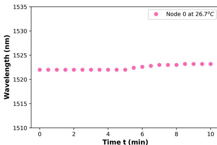
**Figure 12.** The wavelength shift of node 0 for a DCFPI using PDMS in a constant value of a temperature of 26.7 °C.
