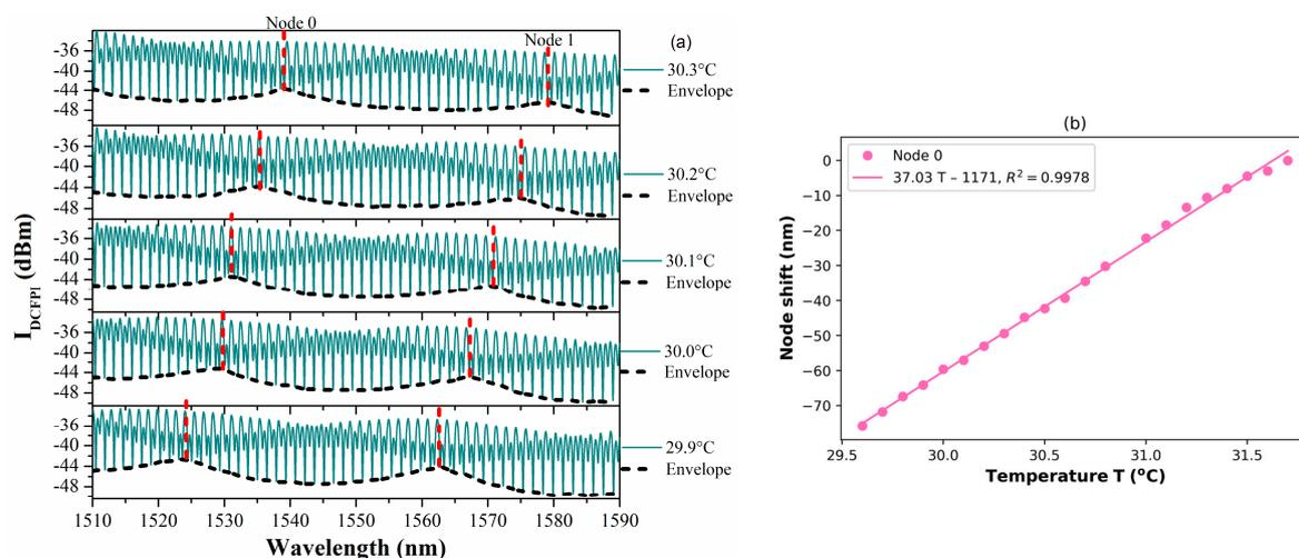
**Figure 7.** (a) Measured spectra of the DCFPI and (b) the characteristic curve of the node wavelength shift in the temperature range of 29.6 to 31.7 °C.
