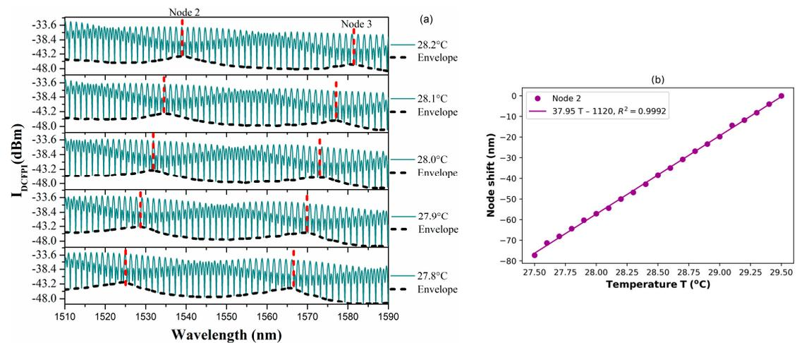
Figure 9. (a) Measured spectra of the DCFPI and (b) the characteristic curve of the node wavelength shift in the temperature range of 27.5 to 29.5 °C.
