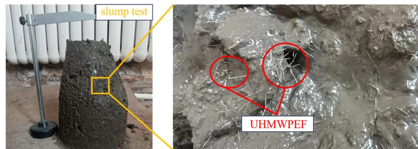
**Figure 3.** Slump test.
